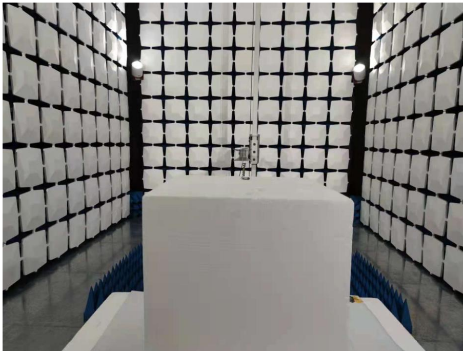
Above 1GHz for radiated emission test setup
