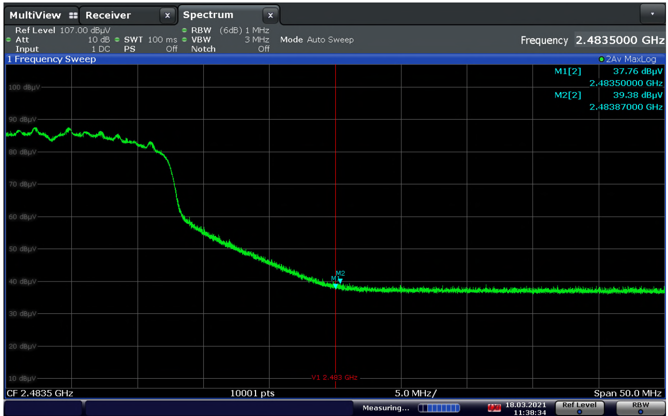
Figure 2-27 – Band-edge, 802.11n HT20 High Channel – Average
