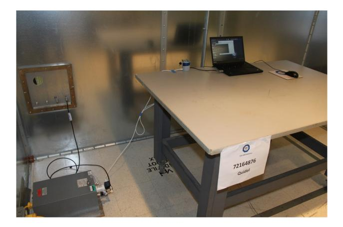
AC Conducted Emissions Test Setup
