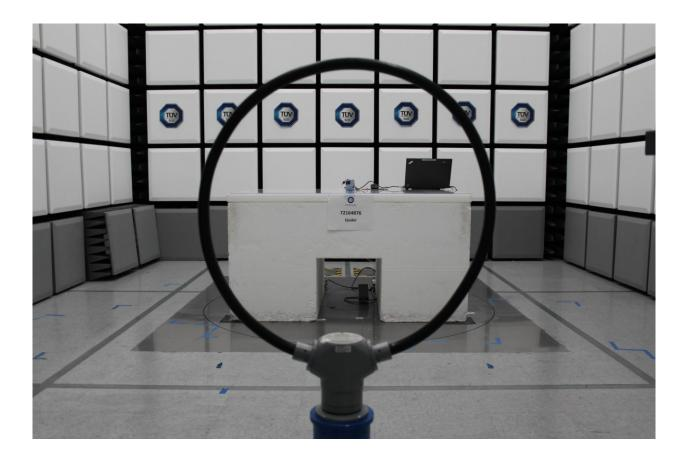
Radiated Emissions Test Setup (Below 30MHz)
