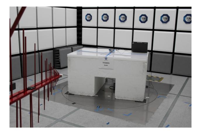
Radiated Emissions Test Setup (30MHz to 1GHz)
