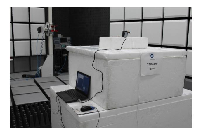
Radiated Emissions Test Setup (1GHz to 18GHz)
