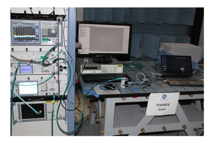
Antenna Conducted Port Test Setup
