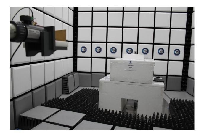
Radiated Emissions Test Setup (Above 18GHz)
