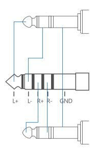
4.4mm balanced to single-ended 3.5mm connections should be made as follows:
