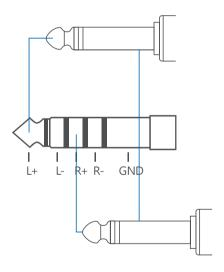
4.4mm balanced to dual stereo 6.3mm connections should be made as follows:
