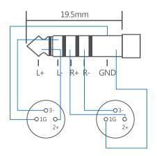
4.4mm balanced to single-ended RCA connections should be made as follows:
