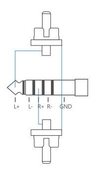
4.4mm balanced to dual mono 6.3mm connections should be made as follows:
