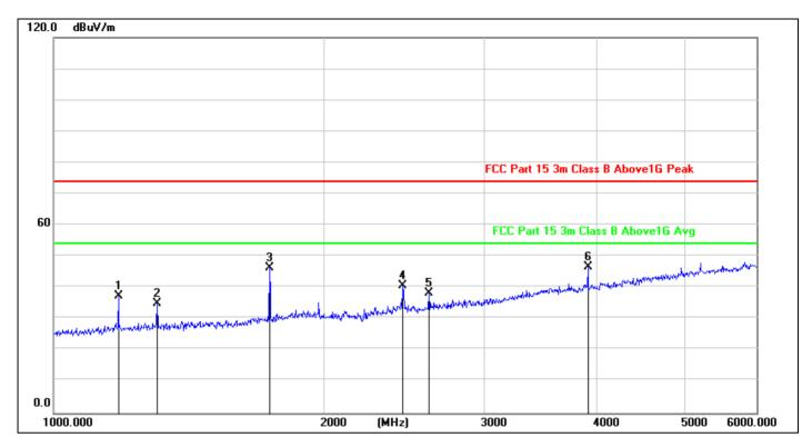
Temperature(C):26(C) Site: LAB Antenna::Vertical Limit: FCC Part 15 C 3m Radiation **Humidity(%):54%** 2022/10/13 21:35:30 **EUT: Automatic Dirt Disposal Test Time: JCB-W2-W01** M/N.: **Power Rating:** AC 120V/60Hz TX **Test Engineer:** Sunshine Mode: Note:
