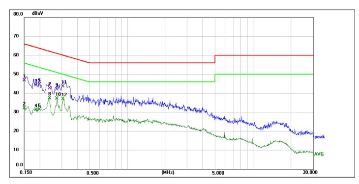
Site:ANCI 843Phase:L1Temperature(C):26(C)Limit:FCC Part 15 Class B Conduction(QP)Humidity(%):54%EUT:Automatic Dirt DisposalTest Time:2022/9/22 21:11:14
