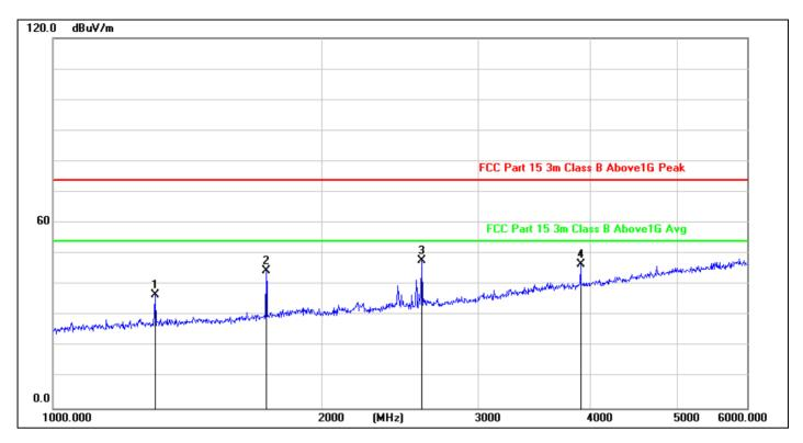
Site: LAB Antenna::Horizontal Temperature(C):26(C) Limit: FCC Part 15 C 3m Radiation **Humidity(%):54%** 2022/10/13 21:34:06 **EUT: Automatic Dirt Disposal Test Time:** JCB-W2-W01 M/N.: **Power Rating:** AC 120V/60Hz TX **Test Engineer:** Sunshine Mode: Note:
