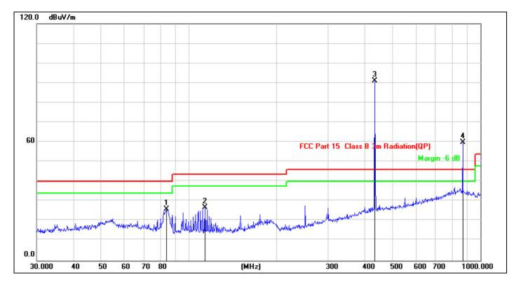
Site: LAB Antenna::Horizontal **Temperature(C):26(C)** Limit: FCC Part 15 C 3m Radiation **Humidity(%):54%** 2022/10/13 21:02:18 **EUT: Automatic Dirt Disposal Test Time:** JCB-W2-W01 M/N.: **Power Rating:** AC 120V/60Hz TX **Test Engineer:** Sunshine Mode: Note:
