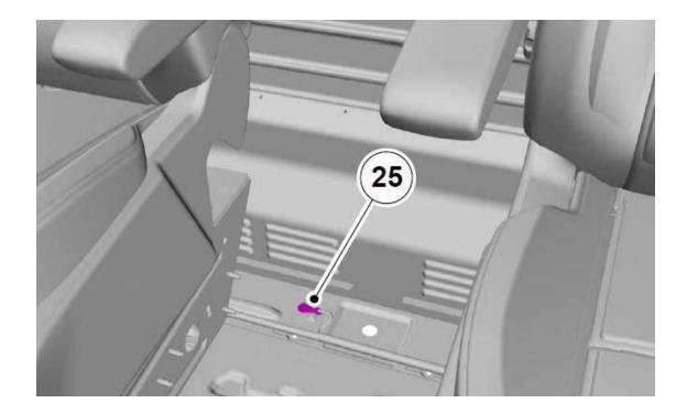
The ignition signal will come from a vehicle-specific connection point. For Ford vehicles it can be reached via the 10-pin connector located under the driver seat. Fleet Edge systems provisioned for Ford Transit vehicles will be shipped to the installer including this connector for quick installation.
