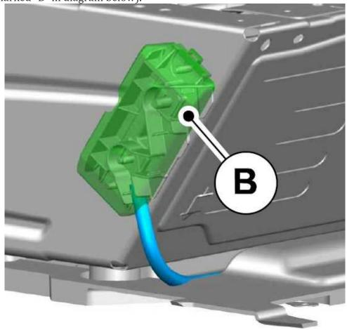
The ground wire will have a similar eyelet connector for connecting to one of the vehicles provided ground studs.
