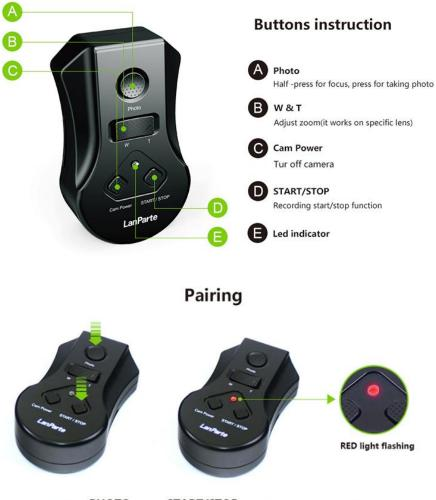
Step1: Hold the "**PHOTO**" and "**START/STOP**" buttons at the same time till the RED LED indicator flashing
