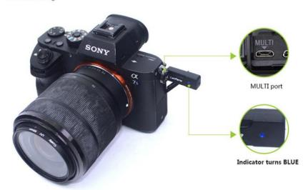
Step2: Plug the receiver into the camera, LED indicator turn **BLUE**, paired.
