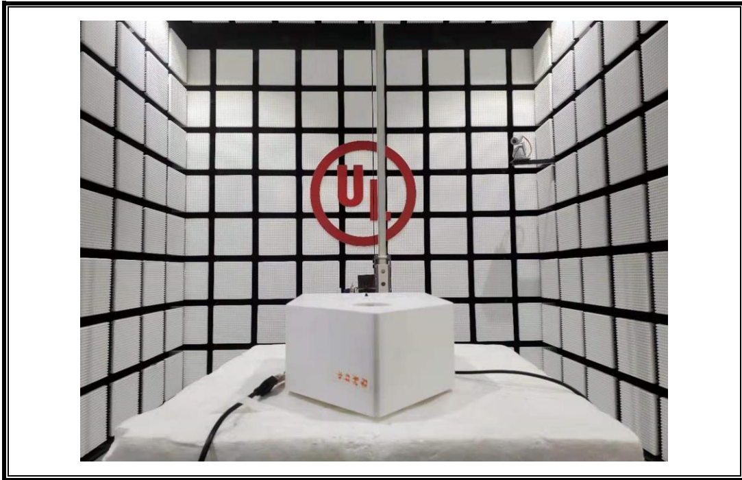
POWERLINE CONDUCTED EMISSIONS MEASUREMENT SETUP
