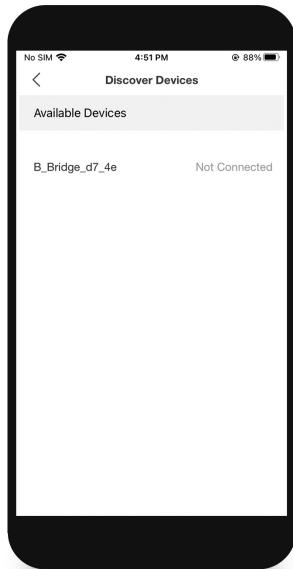
Select the Adapter from the Discover screen, the mobile device will prompt you for a 6-digit code. Plug in the last six digits of your Adapter's serial number, which can be found on the front label of the Adapter. This step is for multifactor authentication and is for security purposes.
