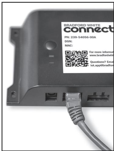
**2.** Plug one end of an ethernet cable into the RJ45 port on the Adapter and another into the RJ45 port on the water heater. Supplied with the Bradford White Connect™ Adapter is a 7 foot CAT5e ethernet cable. Please use either this cable or a similar one, up to a length of 100 feet.
