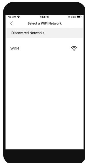
**6.** Once your Adapter and mobile device are connected via Bluetooth, your mobile device will prompt you to select a local wireless network. Select your network and enter the network password using your mobile device.
