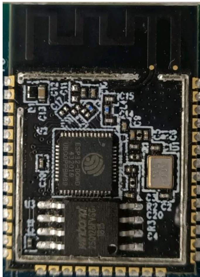
RF Module Close-up view with shield removed
