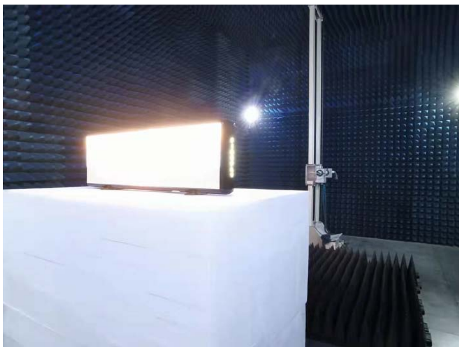
Photo of Radiated Emission Measurement (Above 1G)
