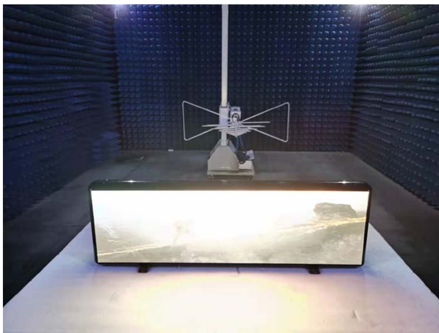
Photo of Radiated Emission Measurement (Below 1G)
