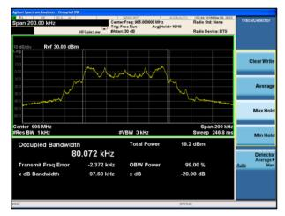
20dB Bandwidth plot on channel 52 (1Mbps)
