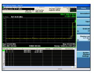
GFSK: Band Edge-High Channel (Hopping Mode)
