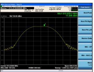
Peak output Power plot on channel 103 (1Mbps)
