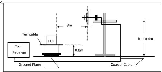
(c) For radiated emissions above 1000MHz
