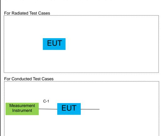
Note: 1. The temporary antenna connector is soldered on the PCB board in order to perform conducted tests and this temporary antenna connector is listed in the equipment list.
