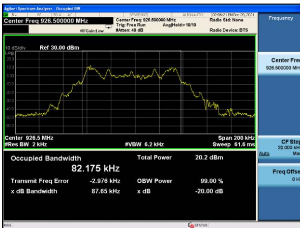
20dB Bandwidth plot on channel 103 (1Mbps)
