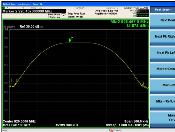
Peak output Power plot on channel 103 (1Mbps)
