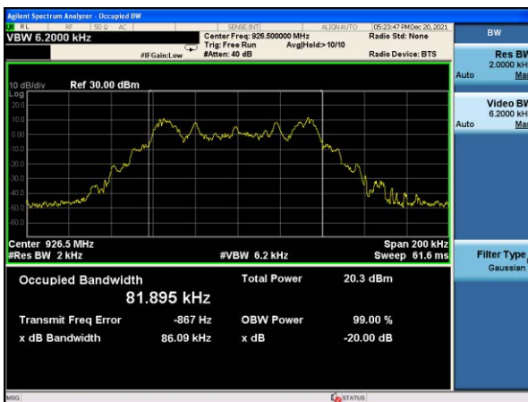
20dB Bandwidth plot on channel 103 (1Mbps)
