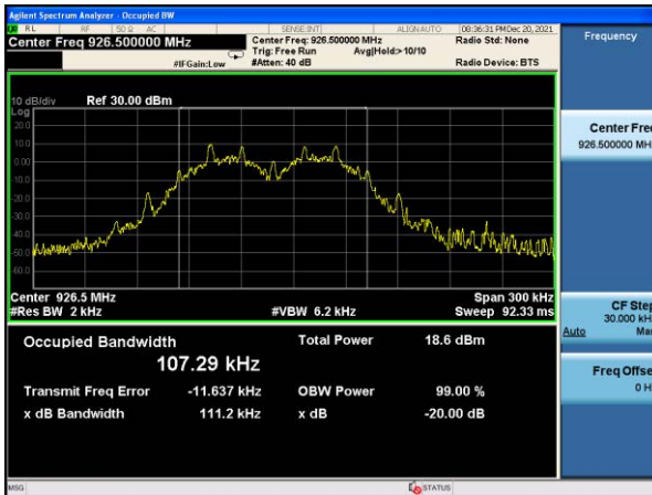
20dB Bandwidth plot on channel 103 (1Mbps)
