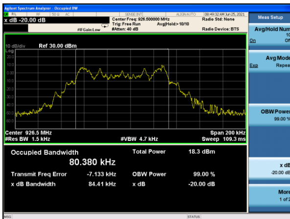
20dB Bandwidth plot on channel 103 (1Mbps)
