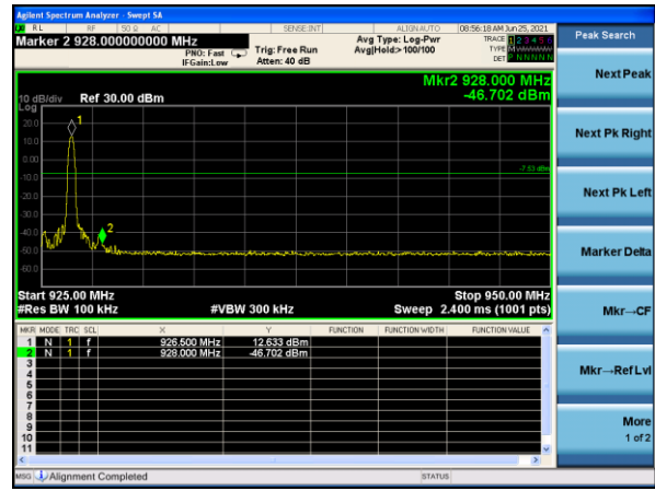
GFSK: Band Edge-High Channel (Hopping Mode)
