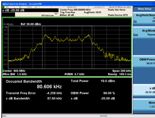
20dB Bandwidth plot on channel 01 (1Mbps)
