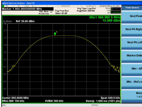
Peak output Power plot on channel 01 (1Mbps)
