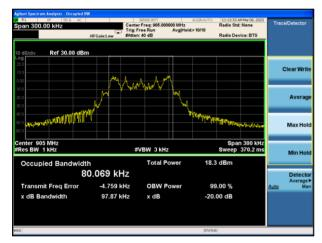
20dB Bandwidth plot on channel 52 (1Mbps)
