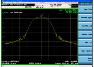
Peak output Power plot on channel 103 (1Mbps)
