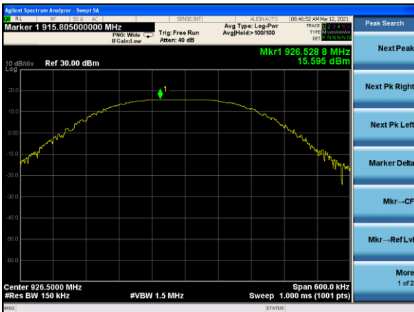
Peak output Power plot on channel 103(1Mbps)
