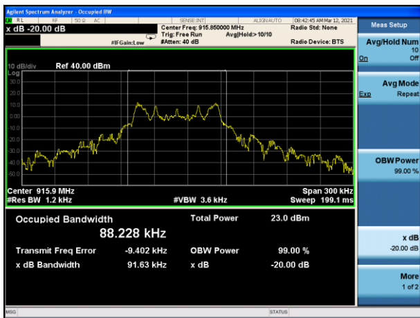
20dB Bandwidth plot on channel 103 (1Mbps)
