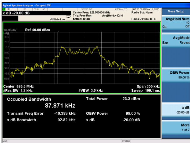
20dB Bandwidth plot on channel 103 (1Mbps)
