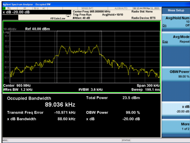
20dB Bandwidth plot on channel 52 (1Mbps)
