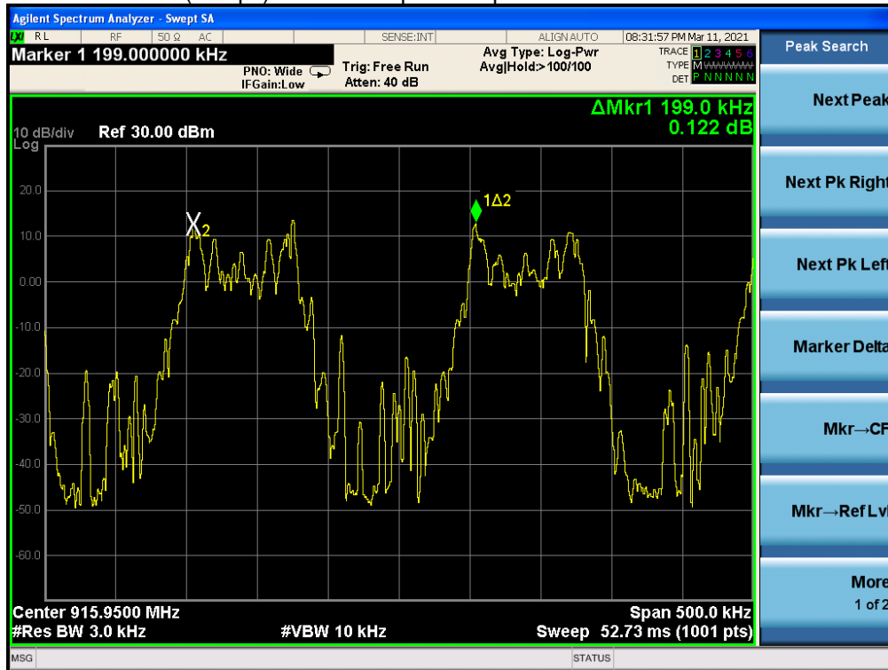
(1Mbps) Channel Separation plot on channel 102-103
