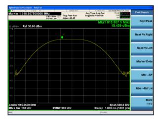
Peak output Power plot on channel 103(1Mbps)
