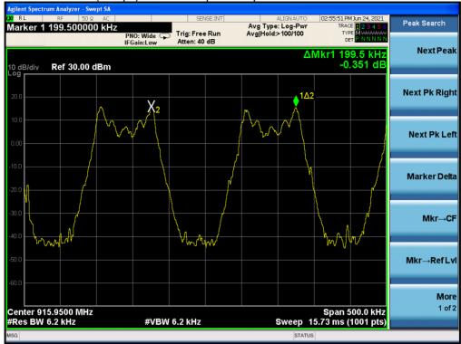
(1Mbps) Channel Separation plot on channel 102-103
