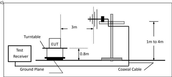
(c) For radiated emissions above 1000MHz
