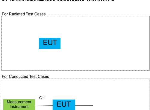
Note: 1. The temporary antenna connector is soldered on the PCB board in order to perform conducted tests and this temporary antenna connector is listed in the equipment list.
