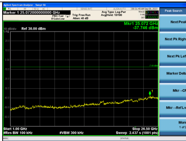
GFSK on channel 103
