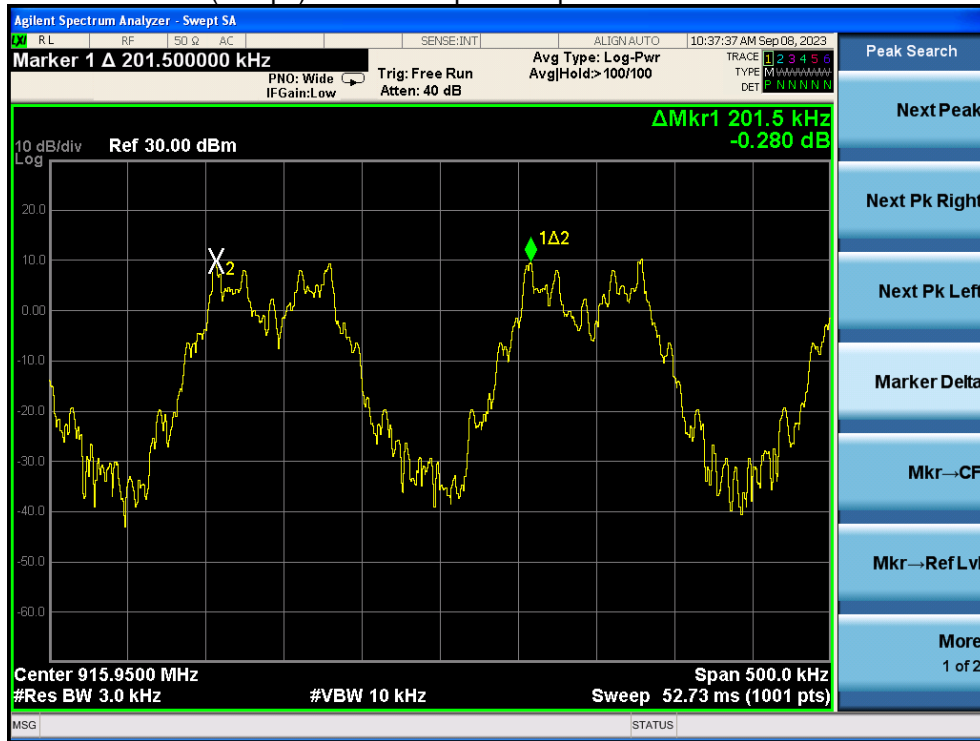
(1Mbps) Channel Separation plot on channel 102-103
