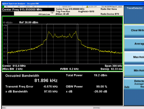
20dB Bandwidth plot on channel 103 (1Mbps)
