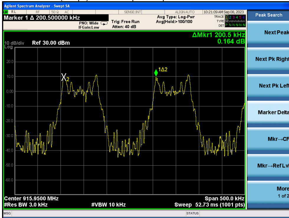
(1Mbps) Channel Separation plot on channel 102-103
