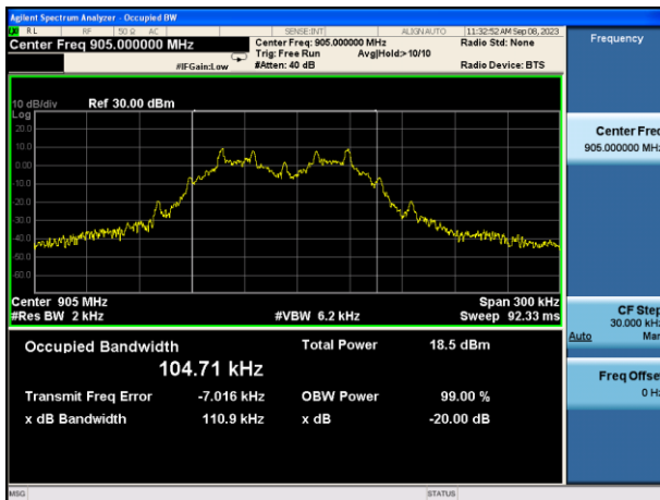
20dB Bandwidth plot on channel 01 (1Mbps)
