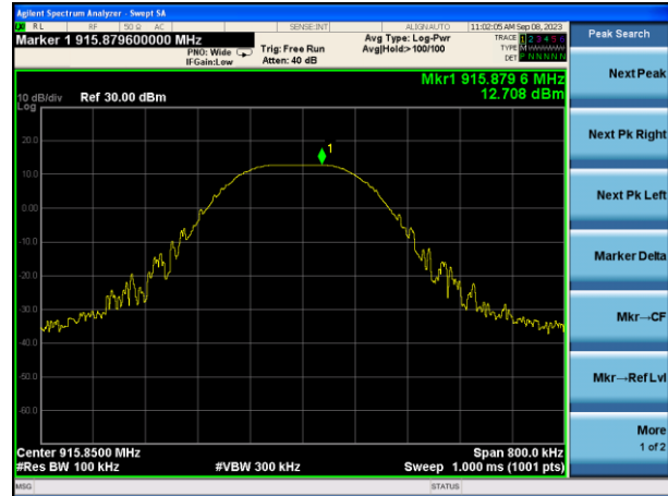
Peak output Power plot on channel 52 (1Mbps)
