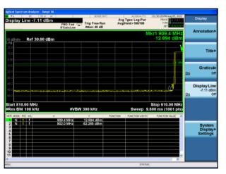
GFSK: Band Edge-High Channel (Hopping Mode)
