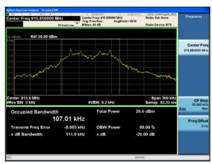
20dB Bandwidth plot on channel 103 (1Mbps)
