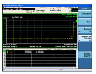
GFSK: Band Edge-High Channel (Hopping Mode)
