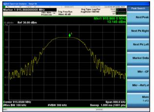
Peak output Power plot on channel 103 (1Mbps)
