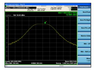
Peak output Power plot on channel 52 (1Mbps)
