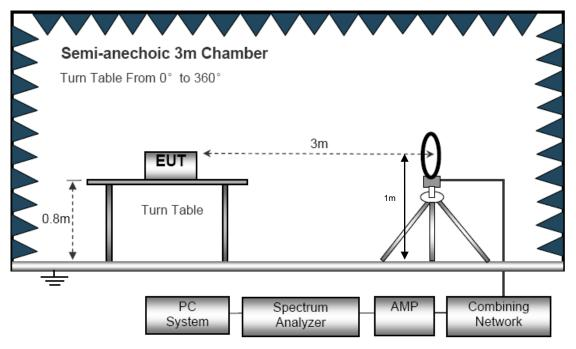
(B) Radiated Emission Test-Up Frequency 30MHz~1GHz
