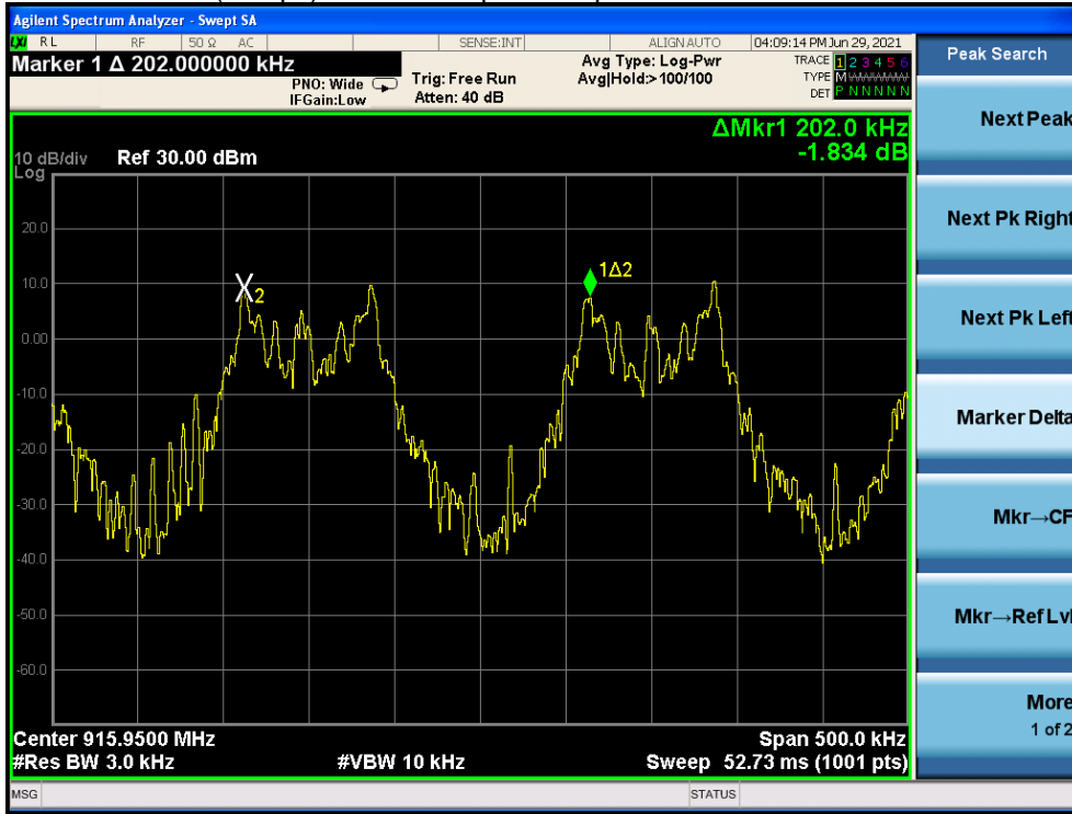
(1Mbps) Channel Separation plot on channel 102-103
