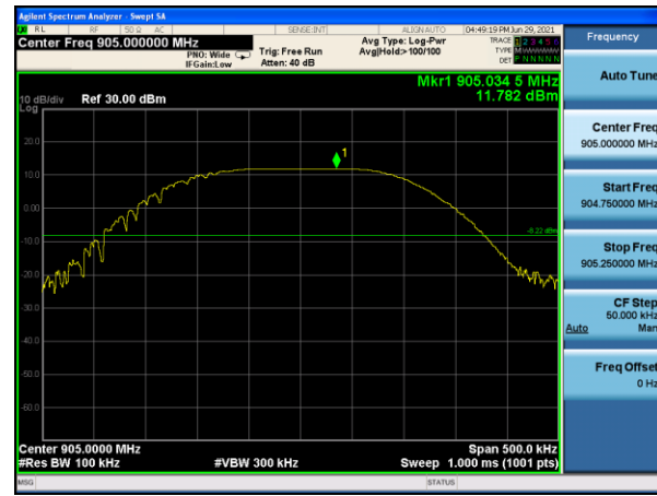
GFSK on channel 01
