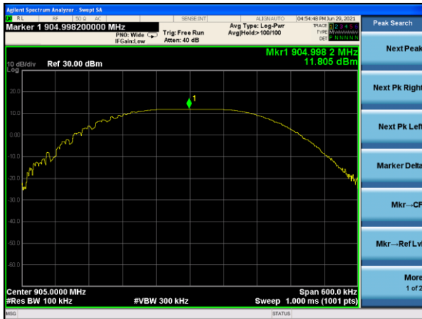
Peak output Power plot on channel 01 (1Mbps)
