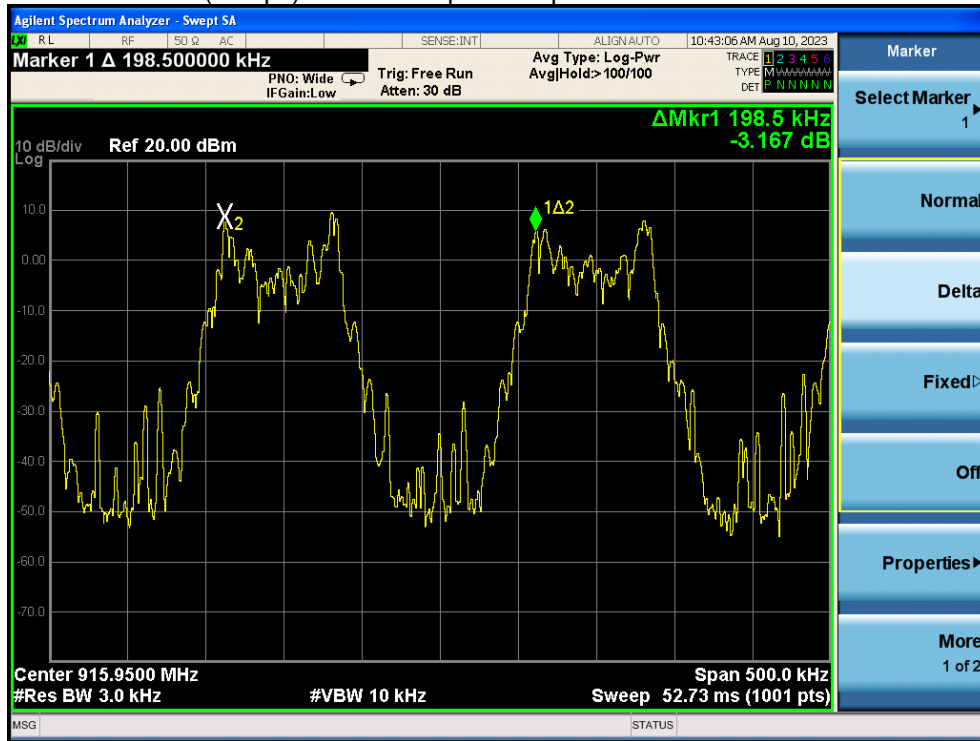
(1Mbps) Channel Separation plot on channel 102-103
