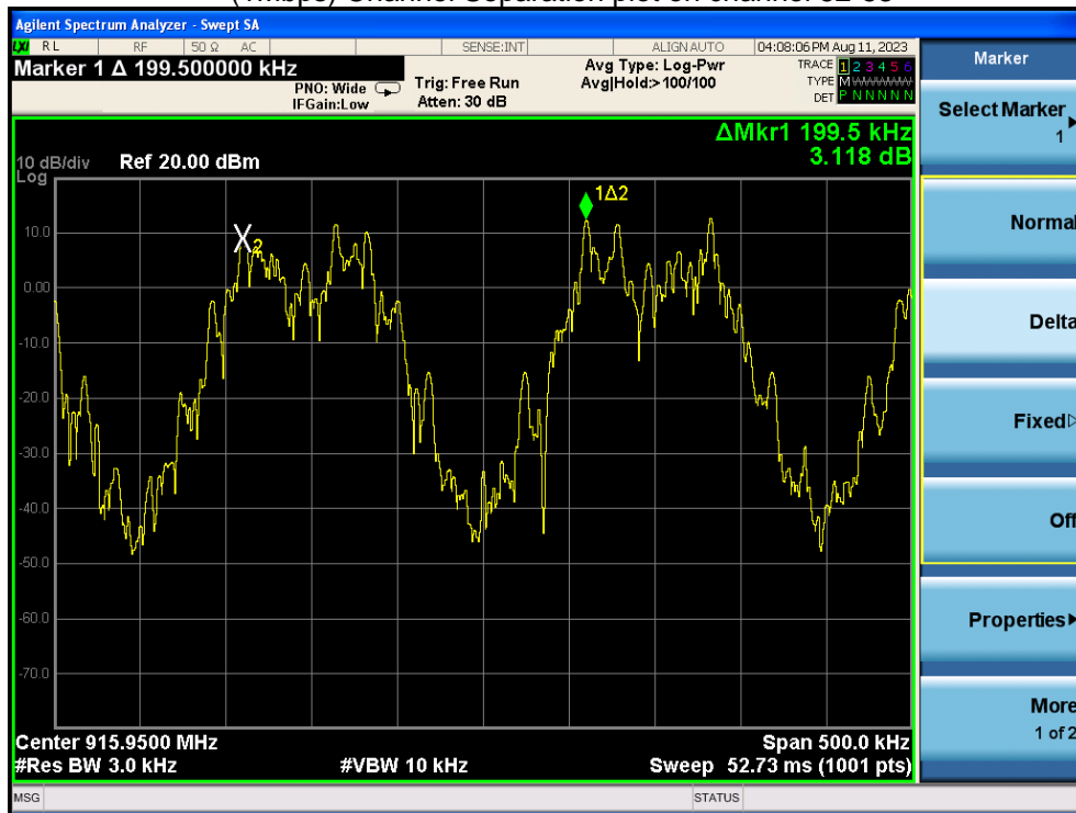
(1Mbps) Channel Separation plot on channel 102-103
