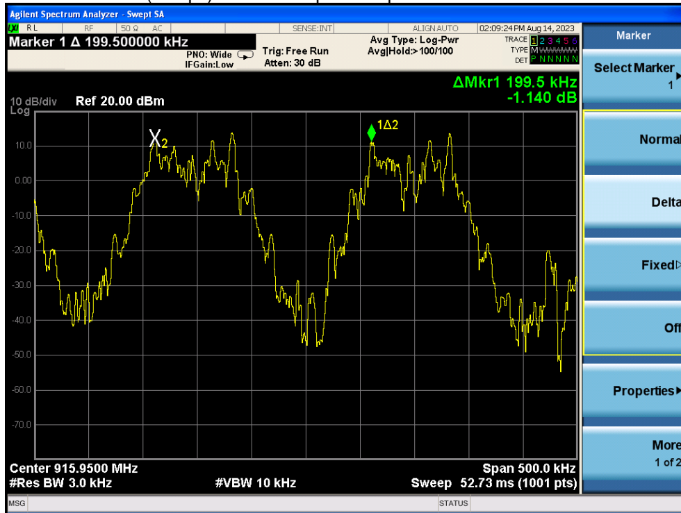
(1Mbps) Channel Separation plot on channel 102-103
