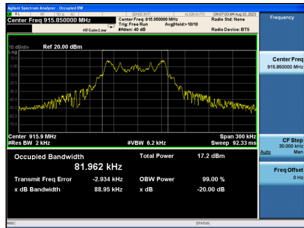
20dB Bandwidth plot on channel 52 (1Mbps)
