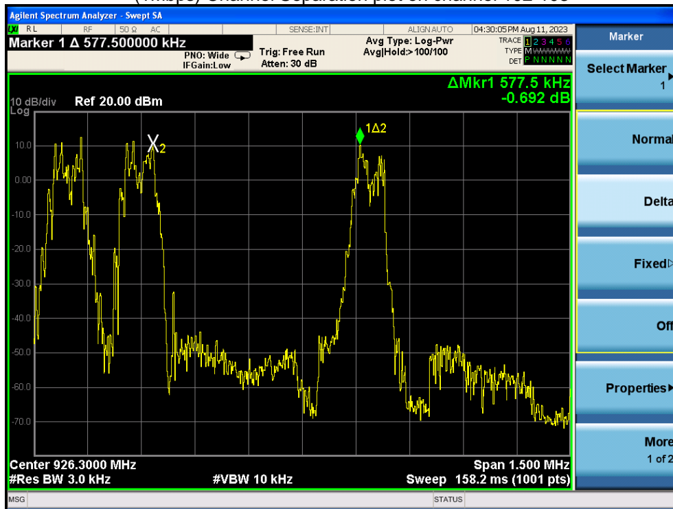
(1Mbps) Channel Separation plot on channel 102-103
