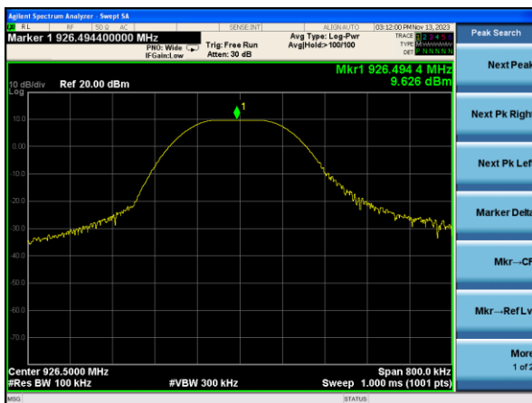
Peak output Power plot on channel 103 (1Mbps)
