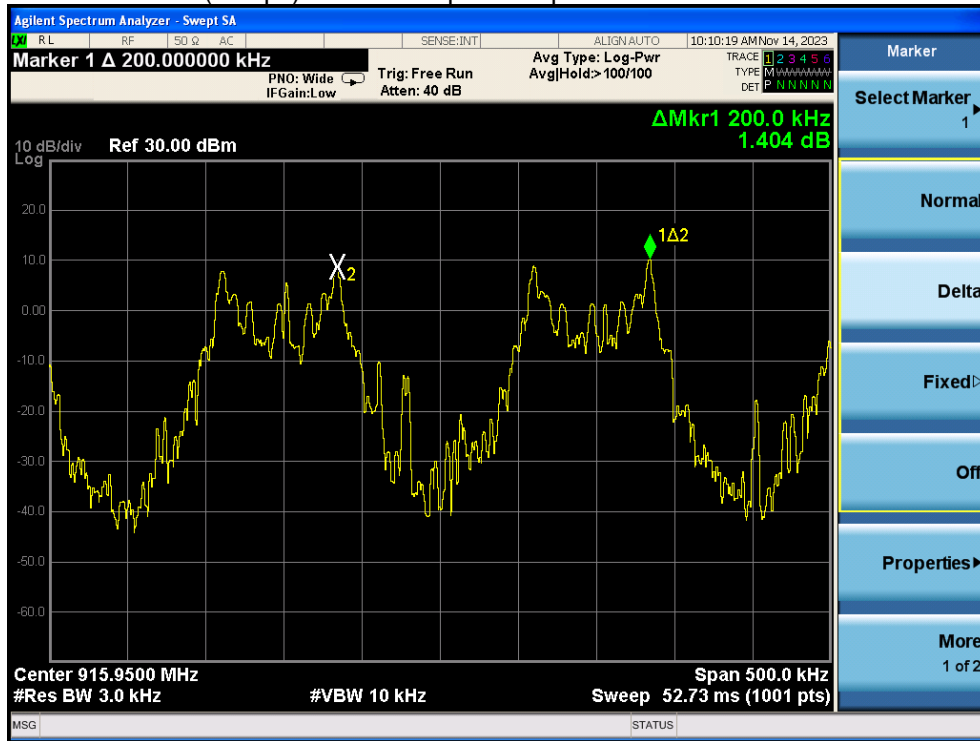
(1Mbps) Channel Separation plot on channel 102-103
