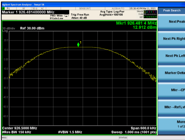
Peak output Power plot on channel 103(1Mbps)
