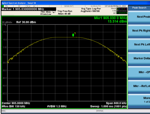
Peak output Power plot on channel 52 (1Mbps)
