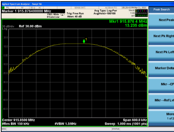
Peak output Power plot on channel 103(1Mbps)
