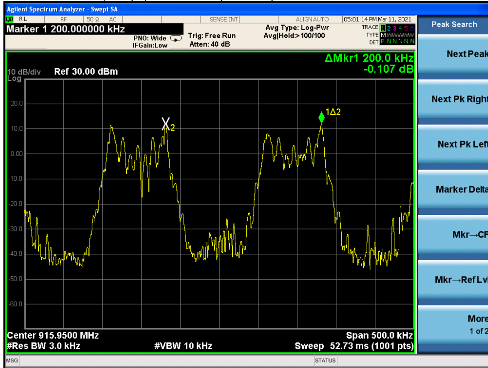
(1Mbps) Channel Separation plot on channel 102-103
