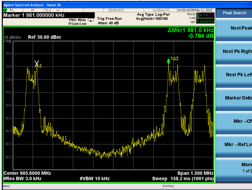
(1Mbps) Channel Separation plot on channel 01-02
