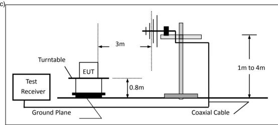
(c) For radiated emissions above 1000MHz
