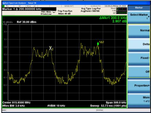
(1Mbps) Channel Separation plot on channel 102-103
