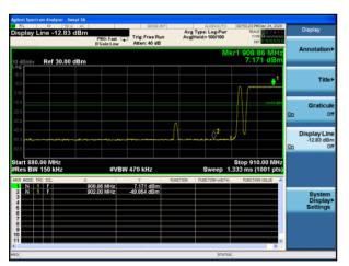
GFSK: Band Edge-High Channel (Hopping Mode)
