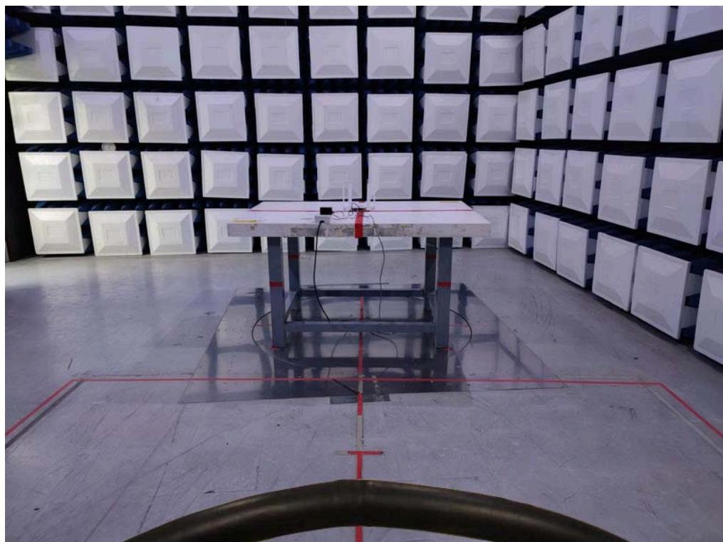
**Radiated Emissions Test Photos****30 MHz to 1 GHz**
