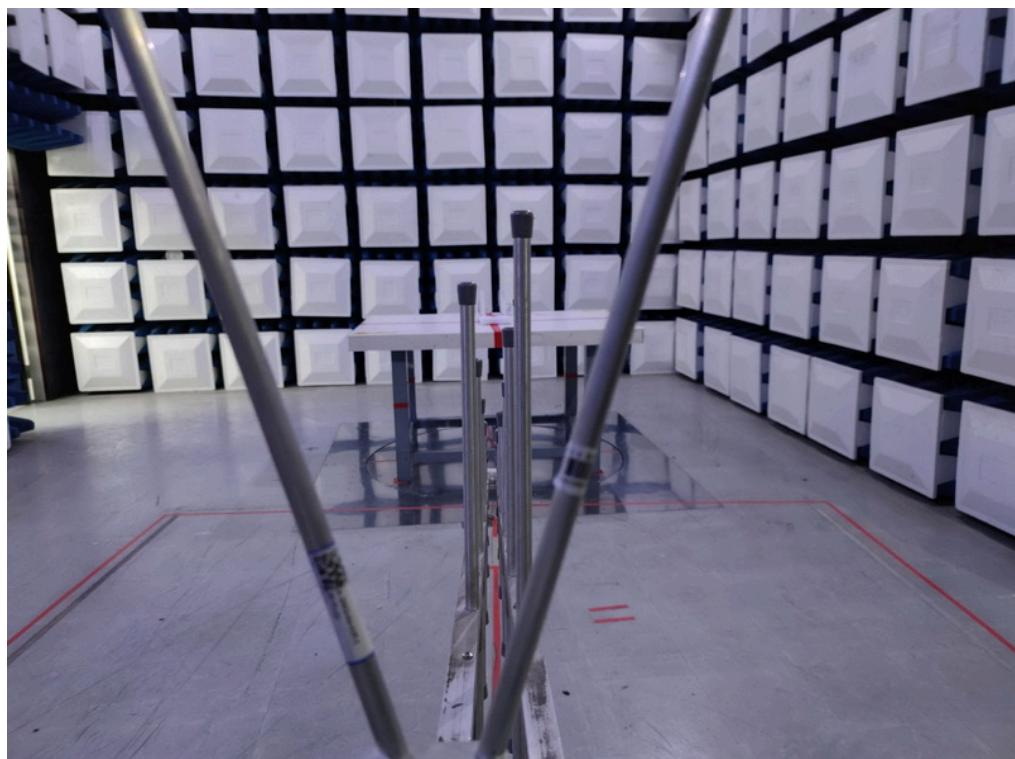
**Radiated Emissions Test Photos****Above 1 GHz**
