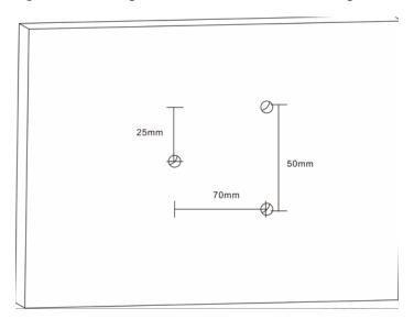
(2) Secure the assembly of the mounting bracket and fiber splice tray to the ceiling or wall by using self-tapping screws and wall anchors.
