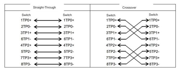
In addition to the preceding cables, the 100BASE-TX/10BASE-T can also use 100-ohm CAT3, CAT4, and CAT5 cables for 10 Mbps, and 100-ohm CAT5 cables for 100 Mbps, both of which support a link length of up to 100 m (328.10 ft). Table 7-2 shows the pinouts of the 100BASE-TX/10BASE-T.
