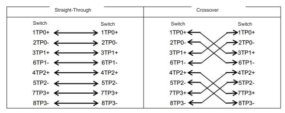
In addition to the preceding cables, the 100BASE-TX can also use 100-ohm CAT3, CAT4, and CAT5 cables for 10 Mbps, and 100-ohm CAT5 cables for 100 Mbps, both of which support a link length of up to 100 m (328.10 ft). Table 7-1 shows the pinouts of the 100BASE-TX.
