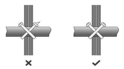
• When cables need to be bent, you should first bundle them up. However, the buckle cannot be bundled within the bend area. Otherwise, considerable stress may be generated in cables, breaking cable cores.
