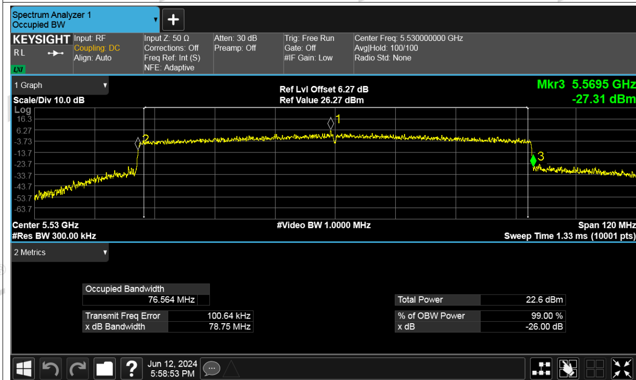
-26dB Bandwidth NVNT be80 5530MHz Ant2
