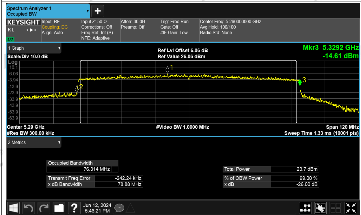
-26dB Bandwidth NVNT be80 5290MHz Ant3
