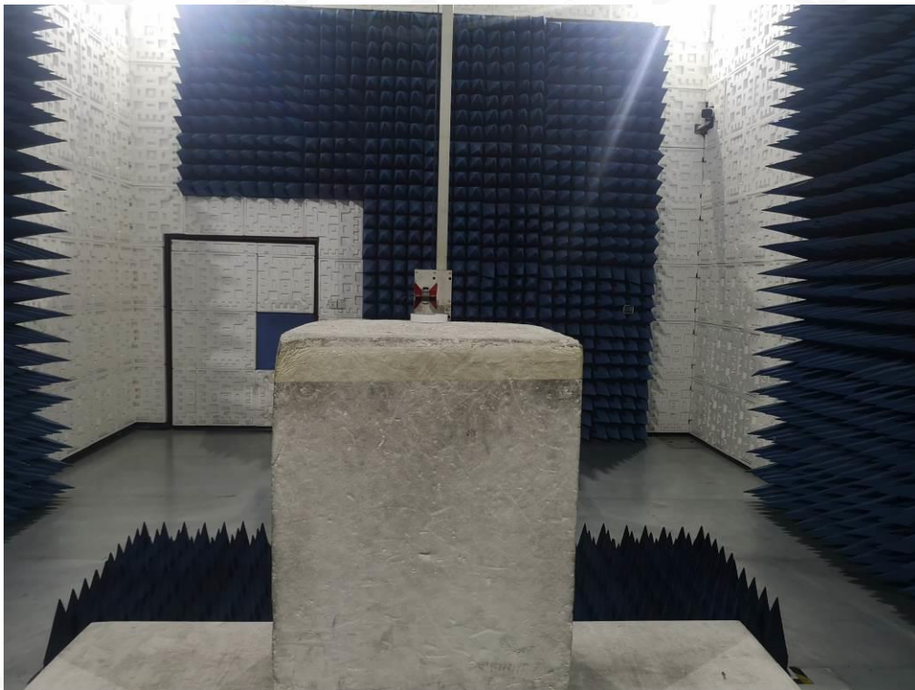
FCC RADIATED EMISSION TEST SETUP ABOVE 1
