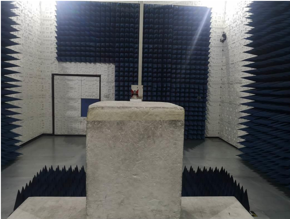
FCC RADIATED EMISSION TEST SETUP ABOVE 1
