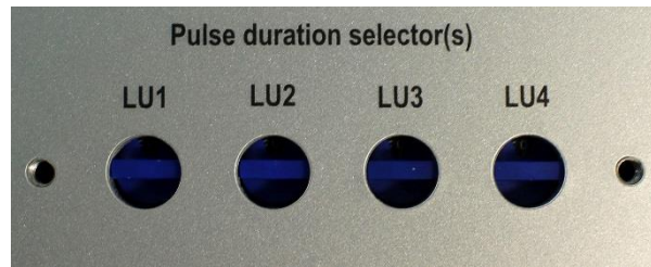
Fig. 3.5. Front panel rotary switches 1...4.
