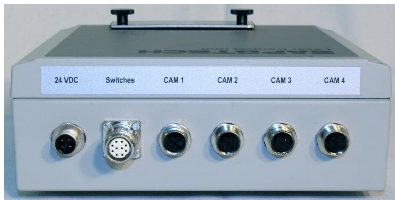
Fig. 3.2. Top panel of CAVILUX OEM control unit.
