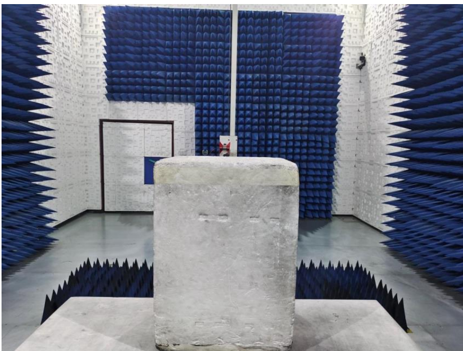
Radiated Emission test setup above 1GHz
