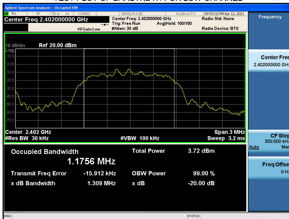
TEST PLOT OF BANDWIDTH FOR LOW CHANNEL
