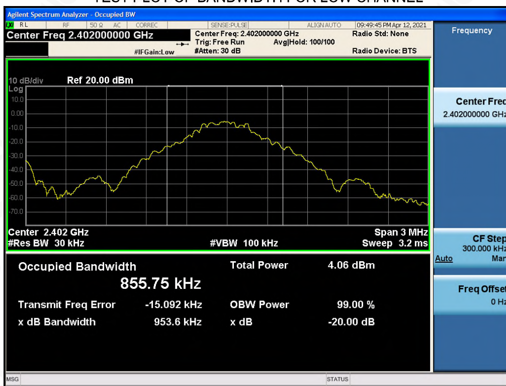
TEST PLOT OF BANDWIDTH FOR LOW CHANNEL
