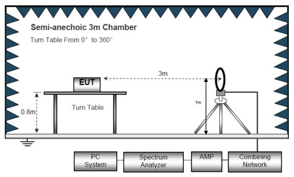
(B) Radiated Emission Test-Up Frequency 30MHz~1GHz
