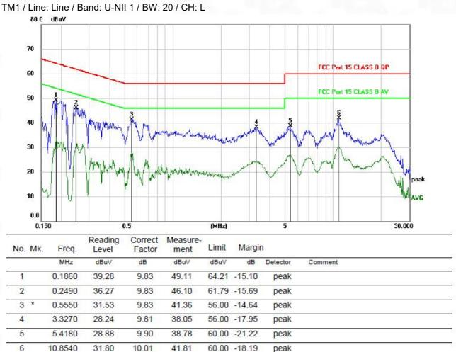
\*:Maximum data x:Over limit I:over margin (Reference Only Note: Measurement=Reading Level+Correc Factor. Factor=(LISN or ISN or PLC or Current Probe)Factor+Cable
