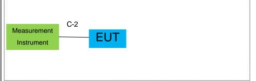
Note:1.The temporary antenna connector is soldered on the PCB board in order to perform conducted tests and this temporary antenna connector is listed in the equipment list.
