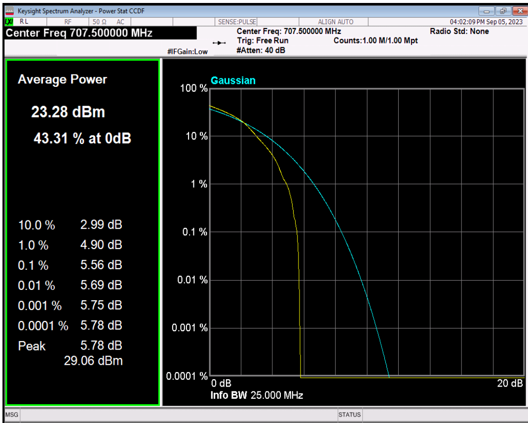
Band12 QPSK BW=10MHz Channel=23095 RB Size=1 Position=#0
