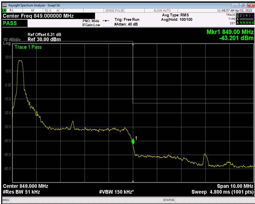
Band5 QAM16 BW=5MHz Channel=20625 RB Size=1 Position=#Max
