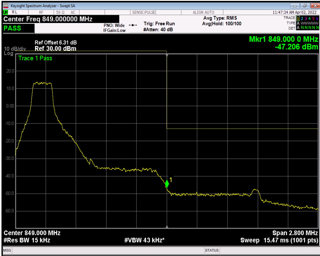
Band5 QPSK BW=1.4MHz Channel=20643 RB Size=1 Position=#Max
