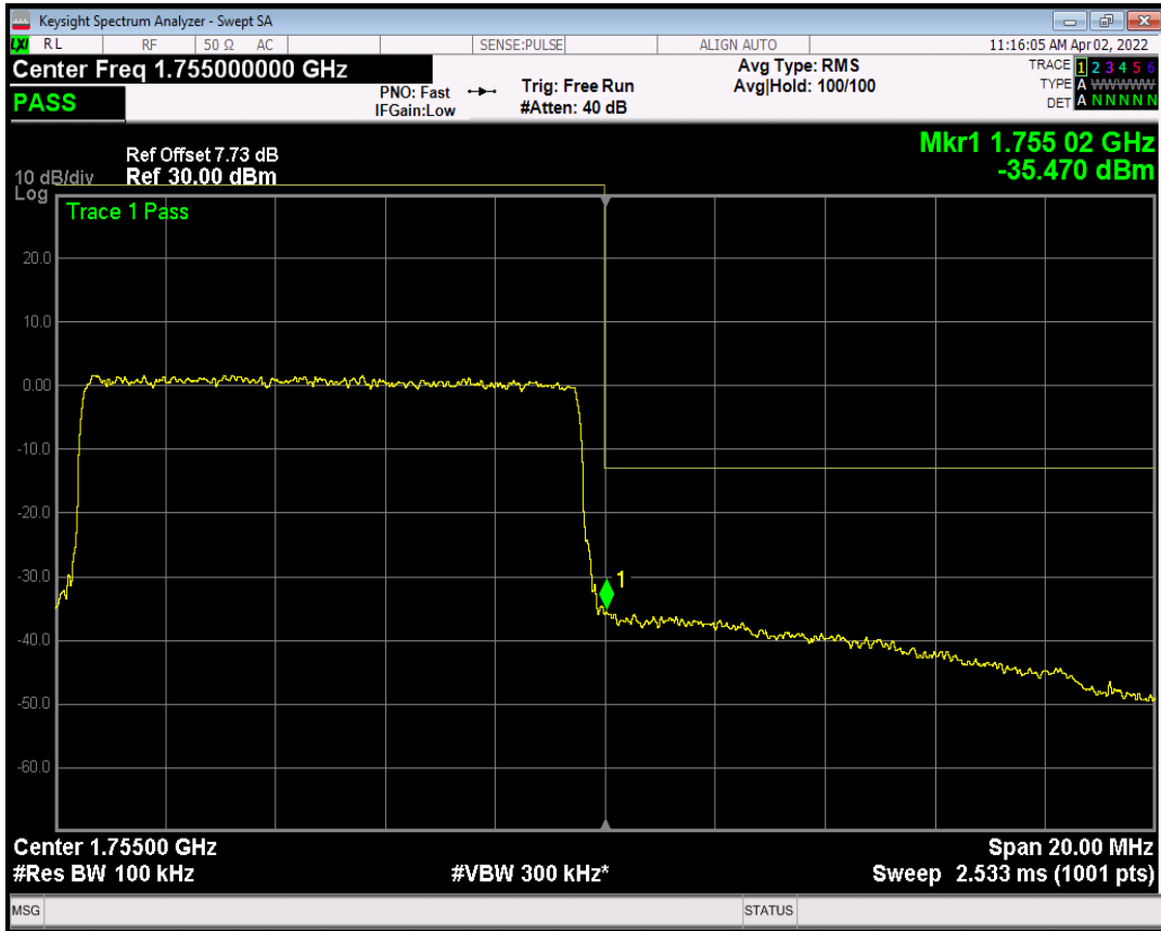
Band4 QPSK BW=15MHz Channel=20025 RB Size=1 Position=#Max
