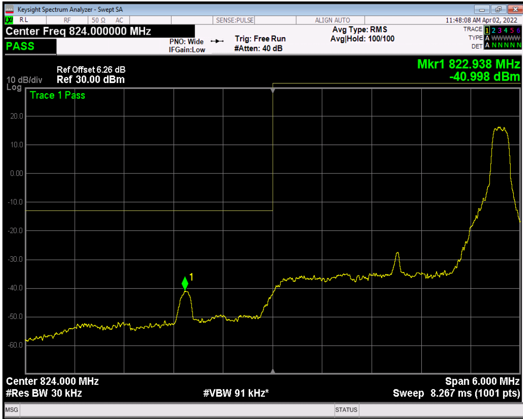
Band5 QAM16 BW=3MHz Channel=20415 RB Size=15 Position=#0
