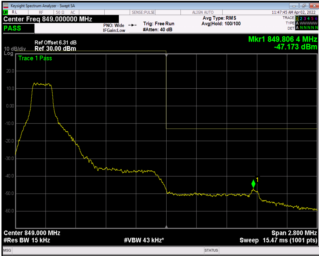
Band5 QPSK BW=1.4MHz Channel=20643 RB Size=6 Position=#0
