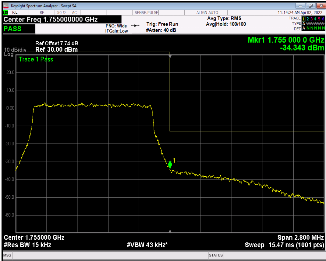
Band4 QPSK BW=3MHz Channel=19965 RB Size=1 Position=#Max
