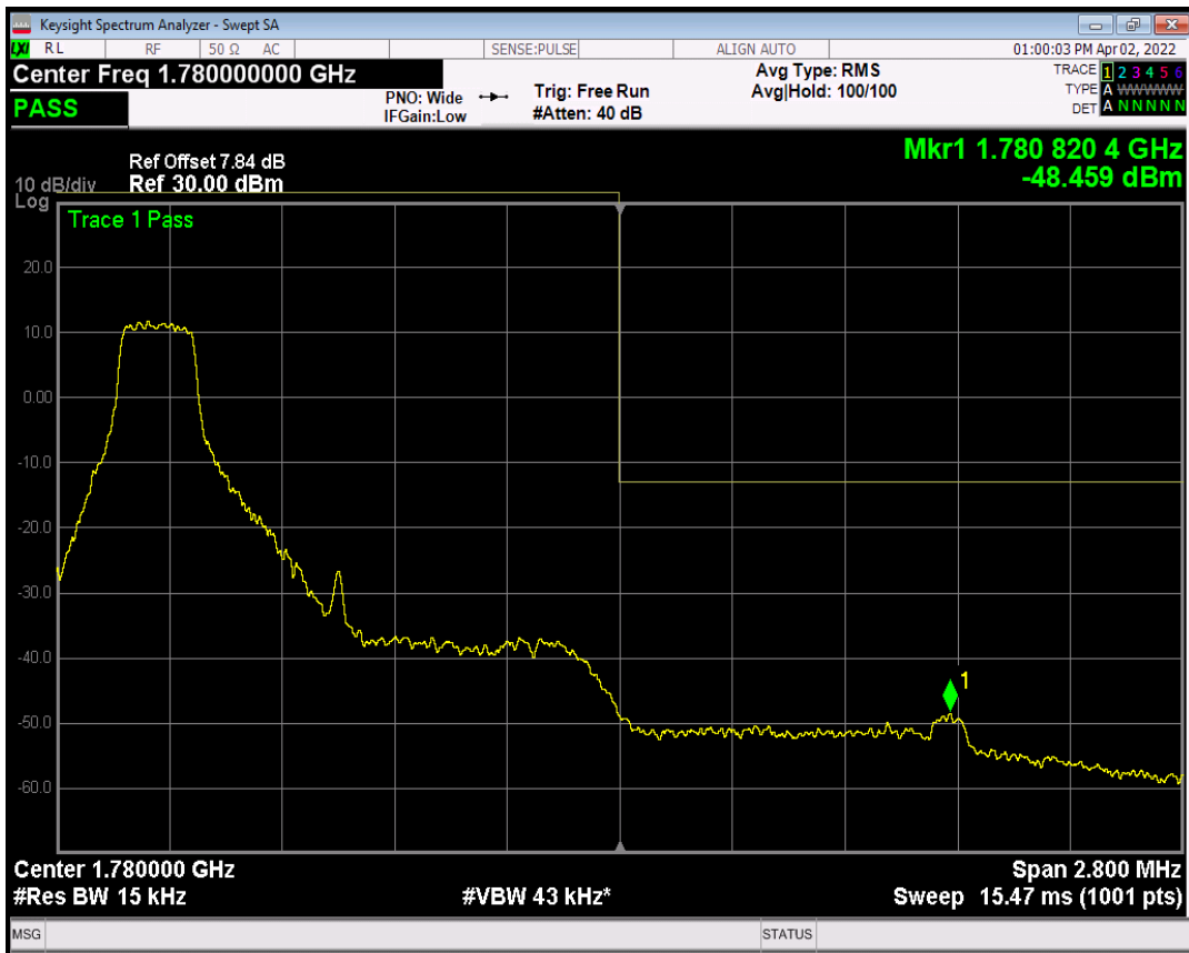
Band66 QAM16 BW=1.4MHz Channel=132665 RB Size=1 Position=#Max
