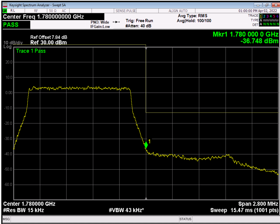
Band66 QAM16 BW=1.4MHz Channel=132665 RB Size=1 Position=#0
