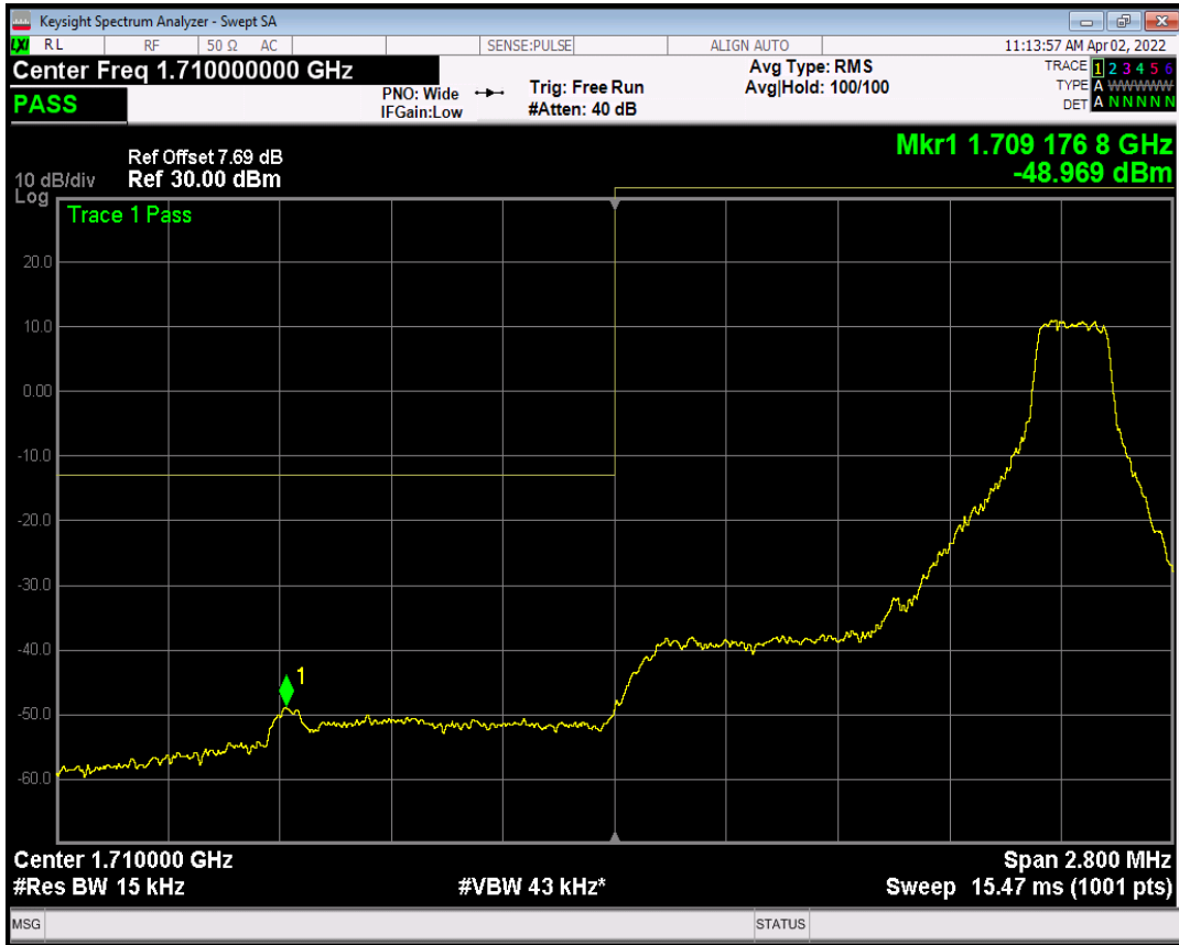
Band4 QAM16 BW=1.4MHz Channel=19957 RB Size=6 Position=#0
