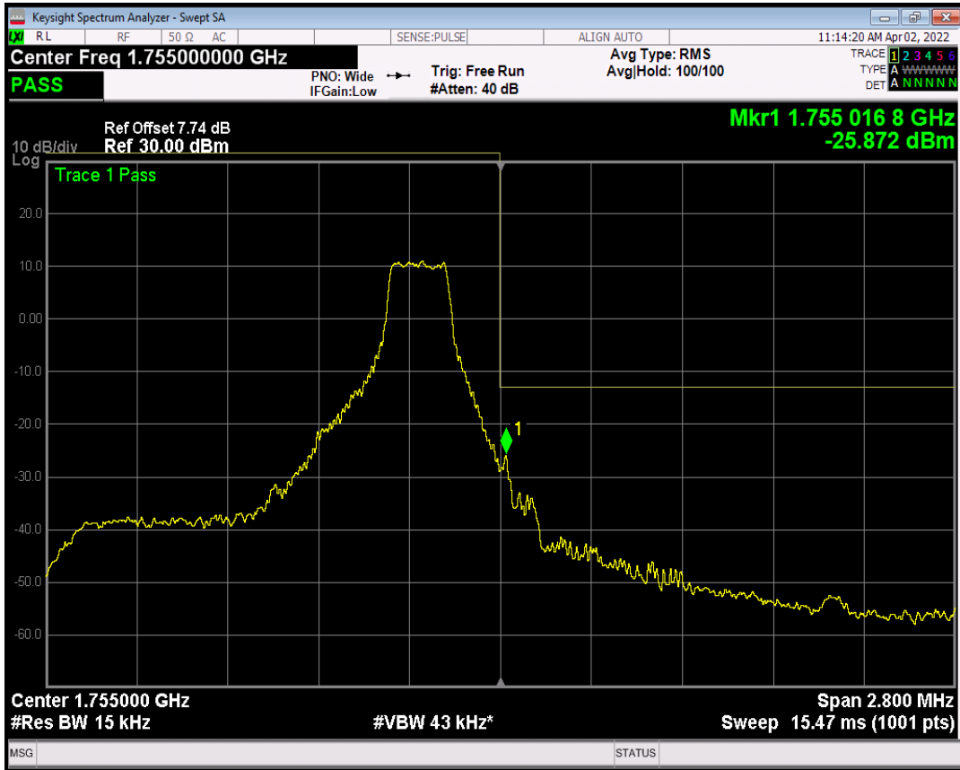
Band4 QPSK BW=3MHz Channel=19965 RB Size=1 Position=#0
