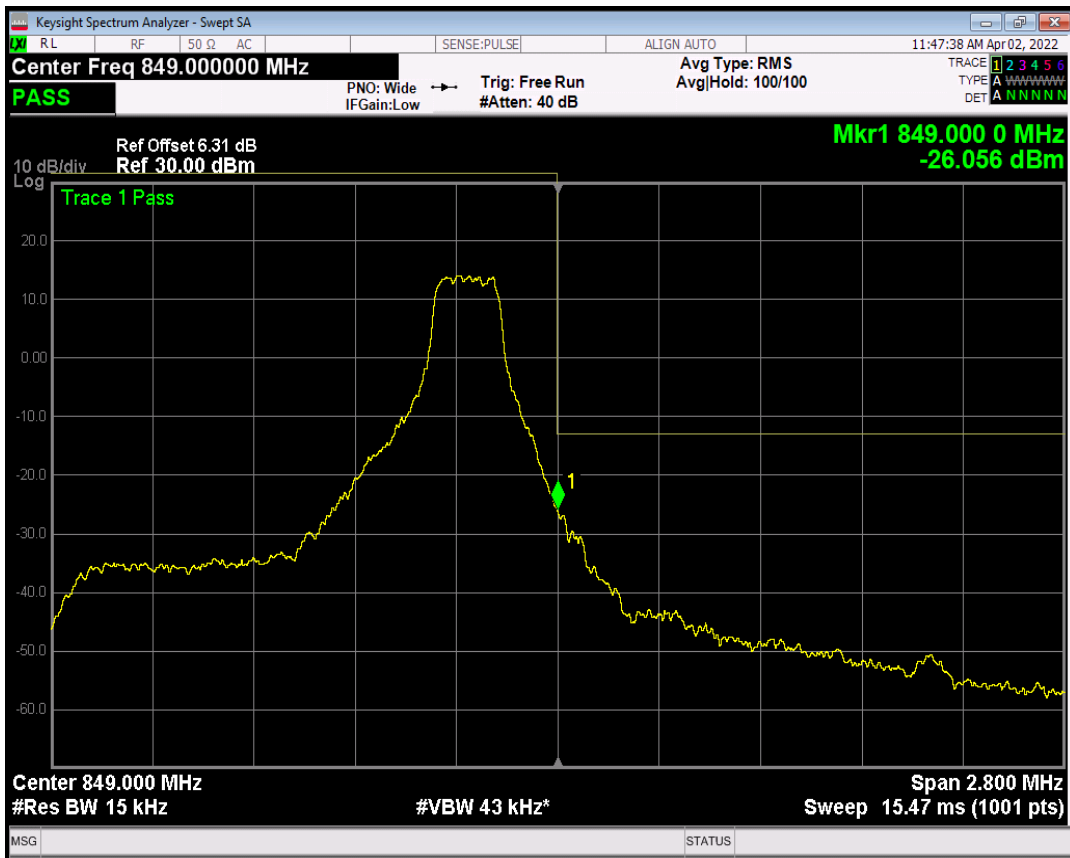
Band5 QAM16 BW=1.4MHz Channel=20643 RB Size=1 Position=#0
