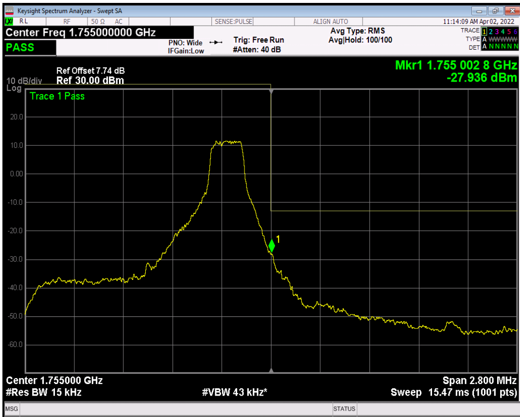
Band4 QPSK BW=1.4MHz Channel=20393 RB Size=6 Position=#0
