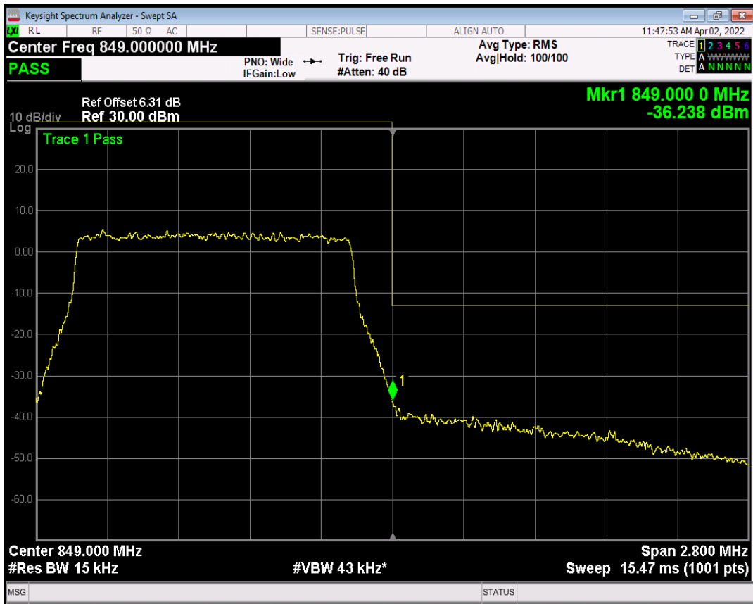
Band5 QPSK BW=3MHz Channel=20415 RB Size=1 Position=#0
