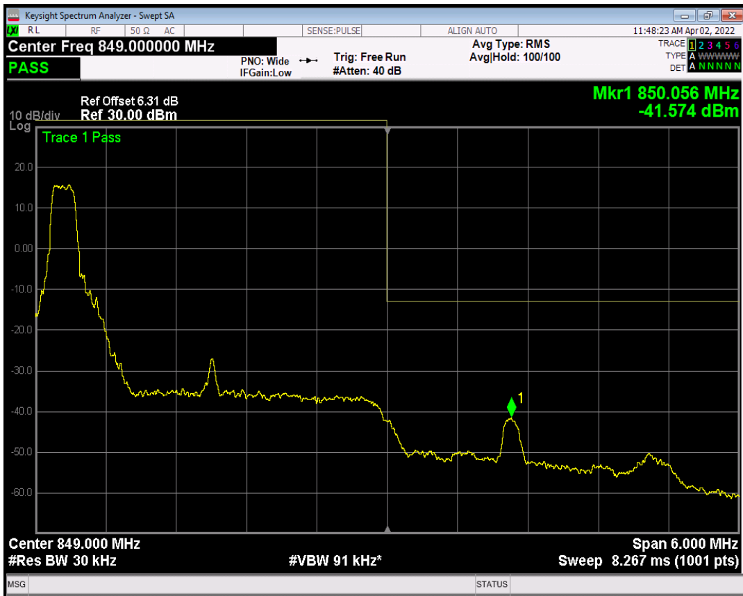
Band5 QAM16 BW=3MHz Channel=20635 RB Size=1 Position=#Max
