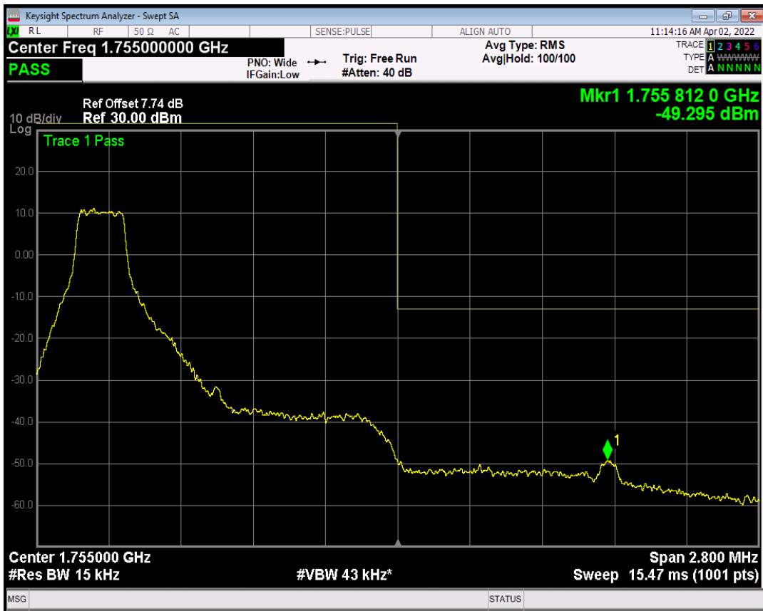
Band4 QAM16 BW=1.4MHz Channel=20393 RB Size=1 Position=#Max
