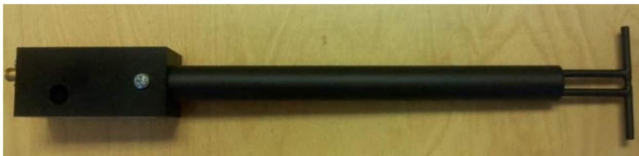
Figure 1 – MVG COMOSAR Validation Dipole
