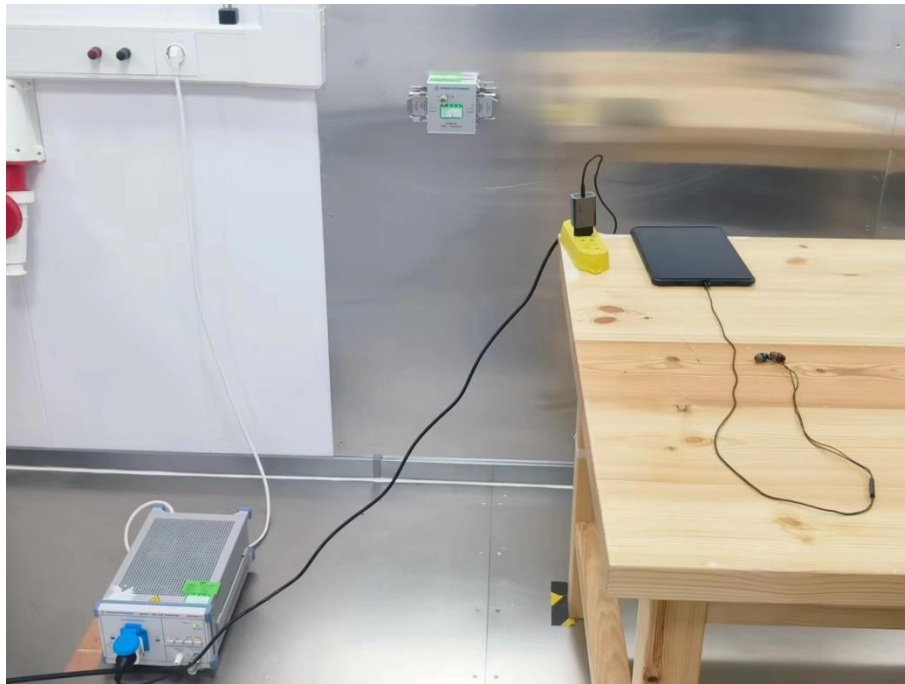
Photographs of the Test Set-up for Conducted Emissions at AC mains power ports
