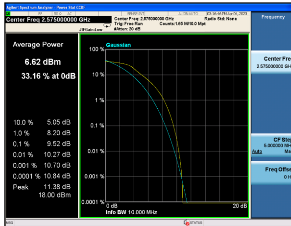
Test Mode: LTE Band 38 Middle channel/20MHz/16-QAM
