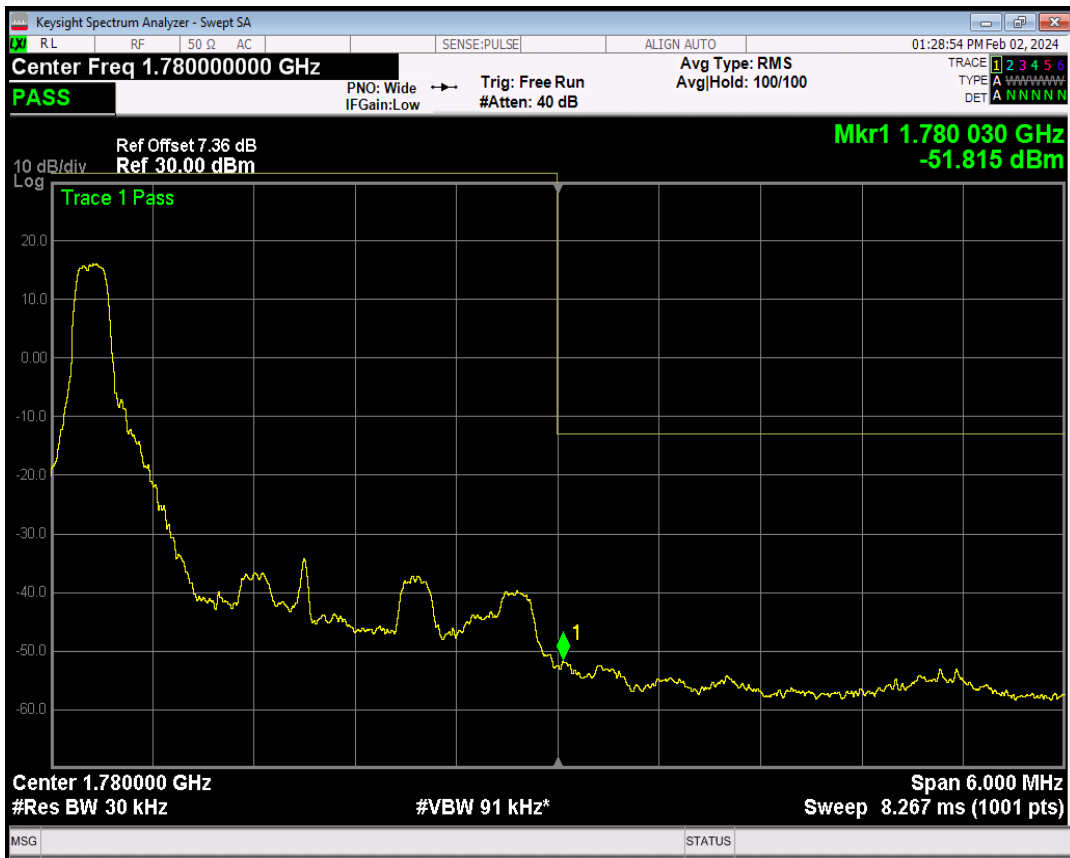
Band66 QPSK BW=3MHz Channel=132657 RB Size=1 Position=#Max
