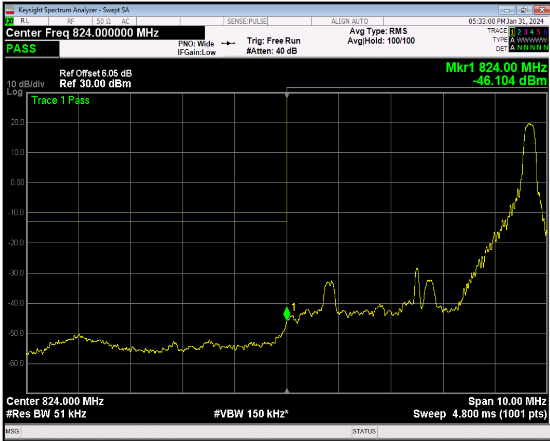
Band5 QPSK BW=5MHz Channel=20425 RB Size=25 Position=#0
