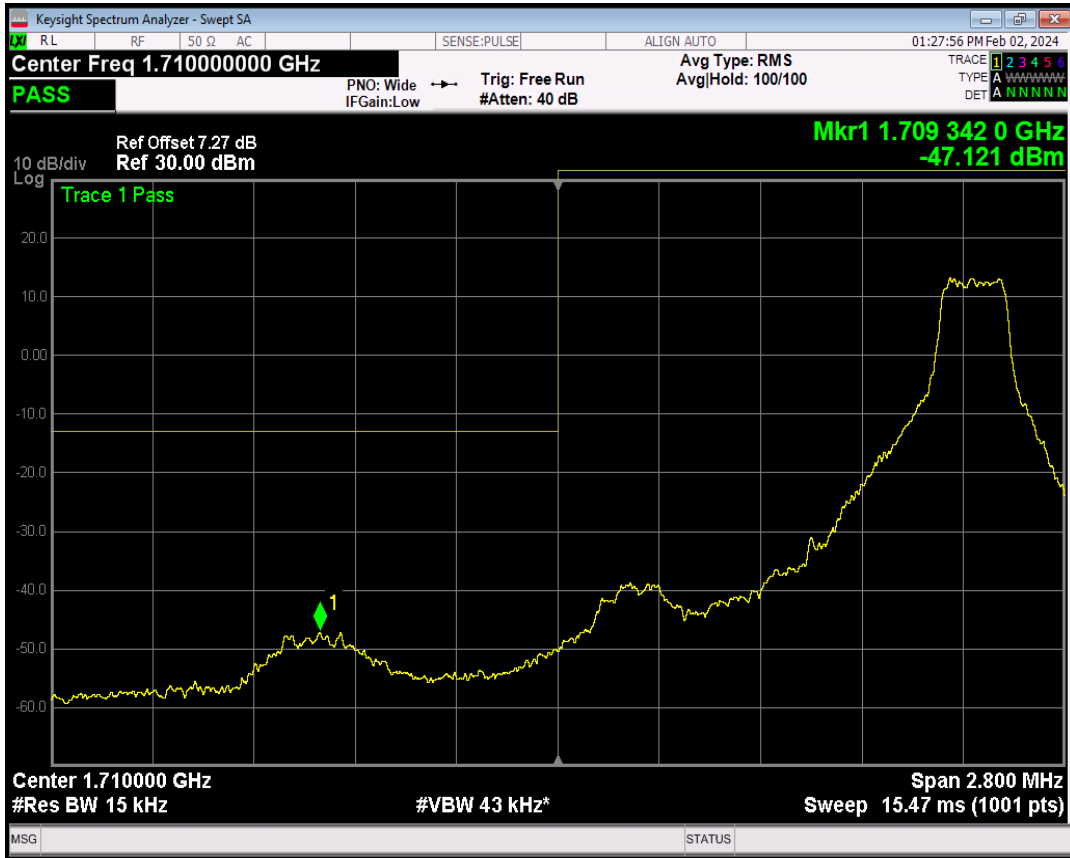
Band66 QPSK BW=1.4MHz Channel=131979 RB Size=6 Position=#0
