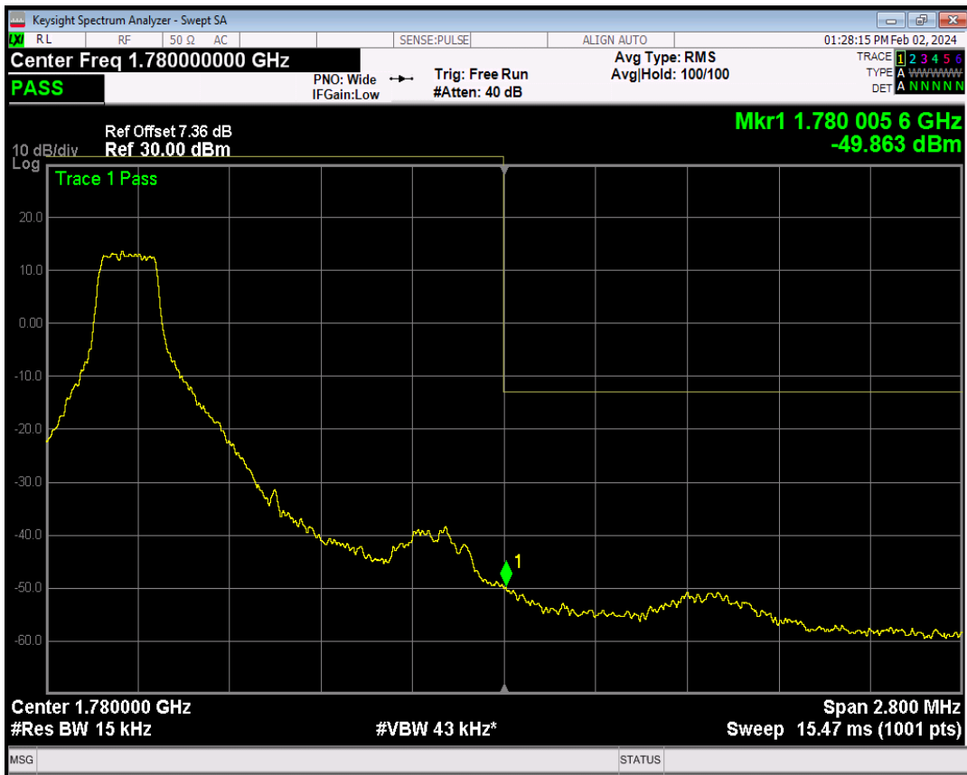
Band66 QPSK BW=1.4MHz Channel=132665 RB Size=1 Position=#Max
