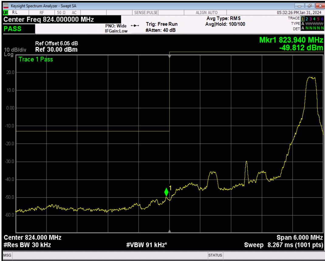
Band5 QPSK BW=3MHz Channel=20415 RB Size=15 Position=#0
