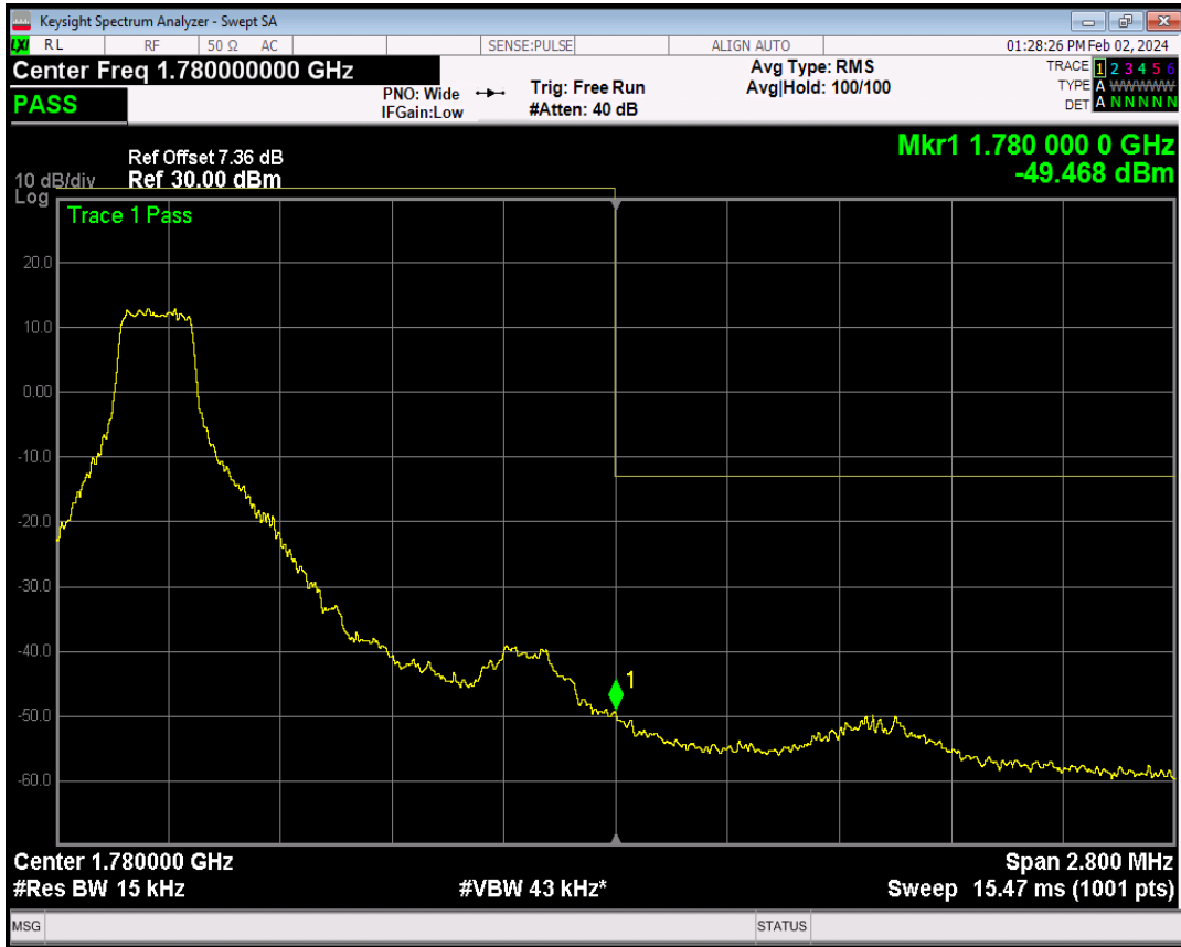
Band66 16QAM BW=1.4MHz Channel=132665 RB Size=1 Position=#Max
