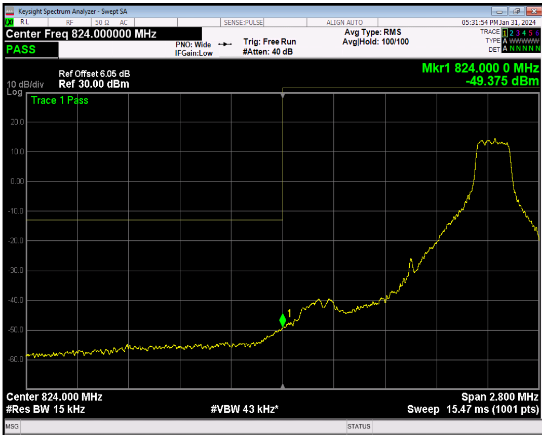
Band5 16QAM BW=1.4MHz Channel=20407 RB Size=6 Position=#0
