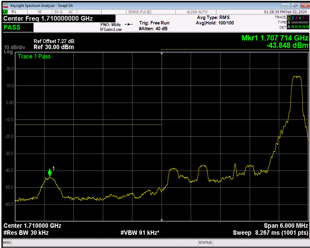
Band66 QPSK BW=3MHz Channel=131987 RB Size=15 Position=#0
