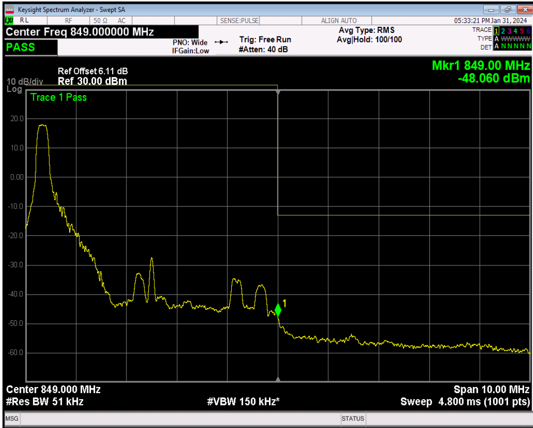
Band5 16QAM BW=5MHz Channel=20625 RB Size=1 Position=#Max
