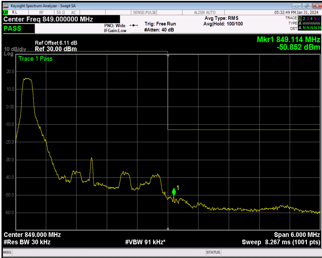
Band5 16QAM BW=3MHz Channel=20635 RB Size=1 Position=#Max
