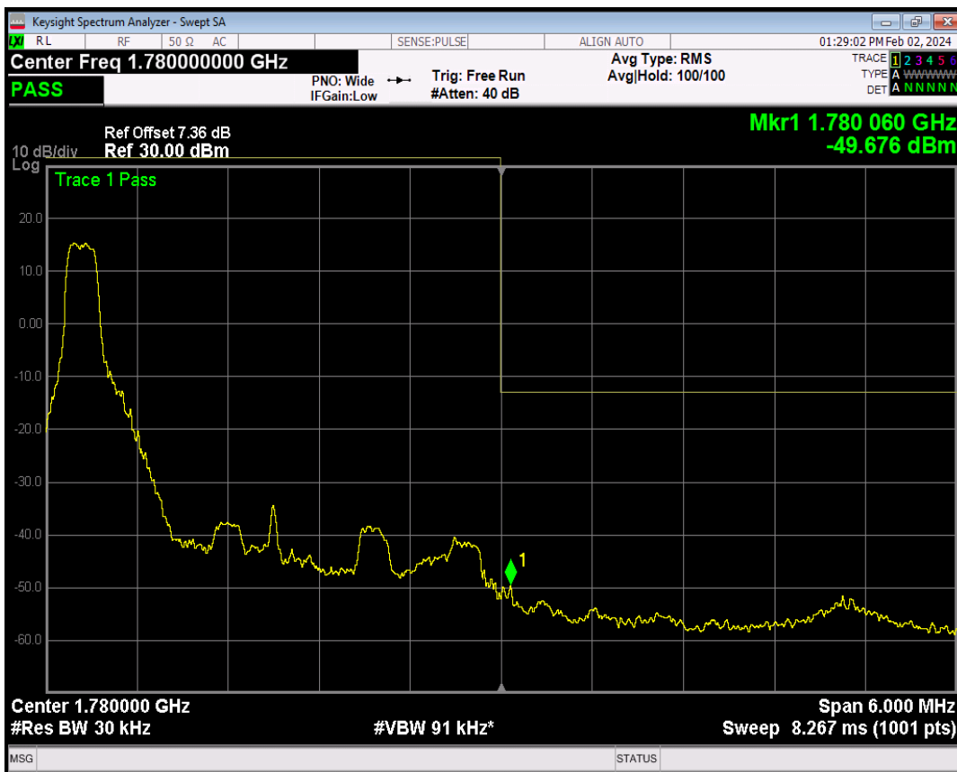
Band66 16QAM BW=3MHz Channel=132657 RB Size=1 Position=#Max
