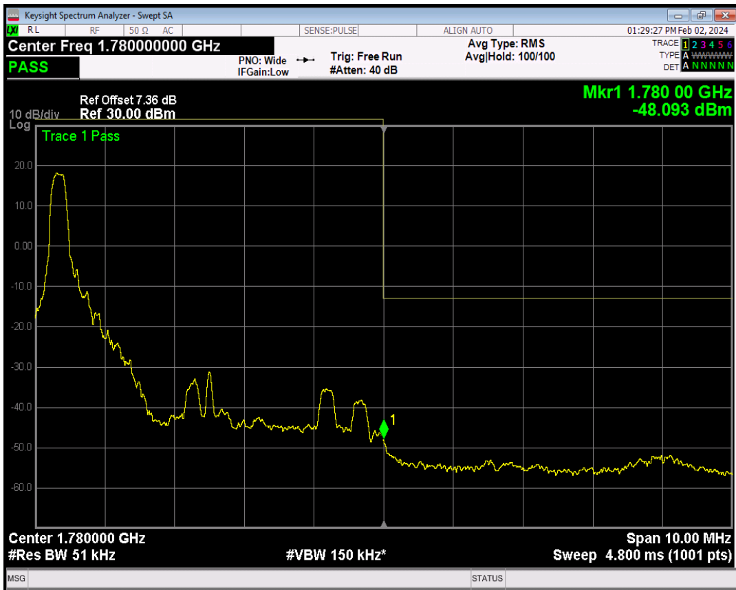
Band66 QPSK BW=5MHz Channel=132647 RB Size=1 Position=#Max
