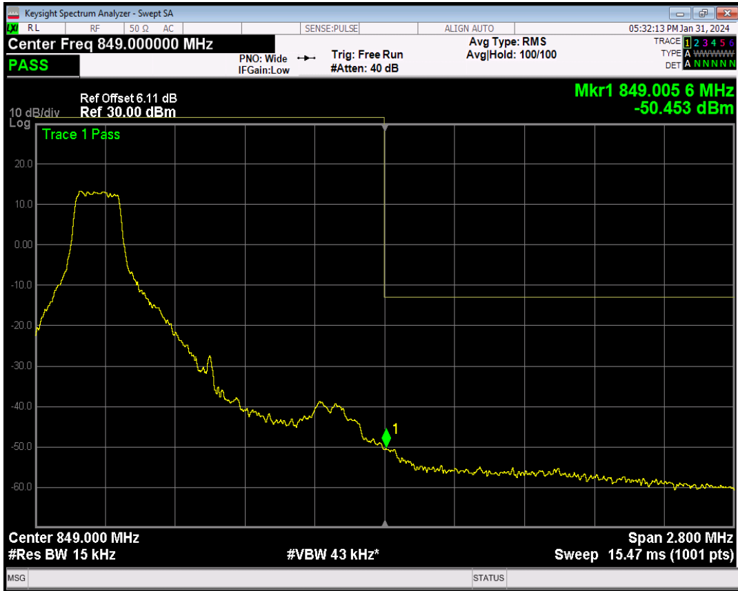
Band5 16QAM BW=1.4MHz Channel=20643 RB Size=1 Position=#Max
