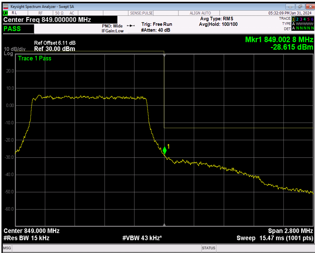
Band5 16QAM BW=1.4MHz Channel=20643 RB Size=1 Position=#0
