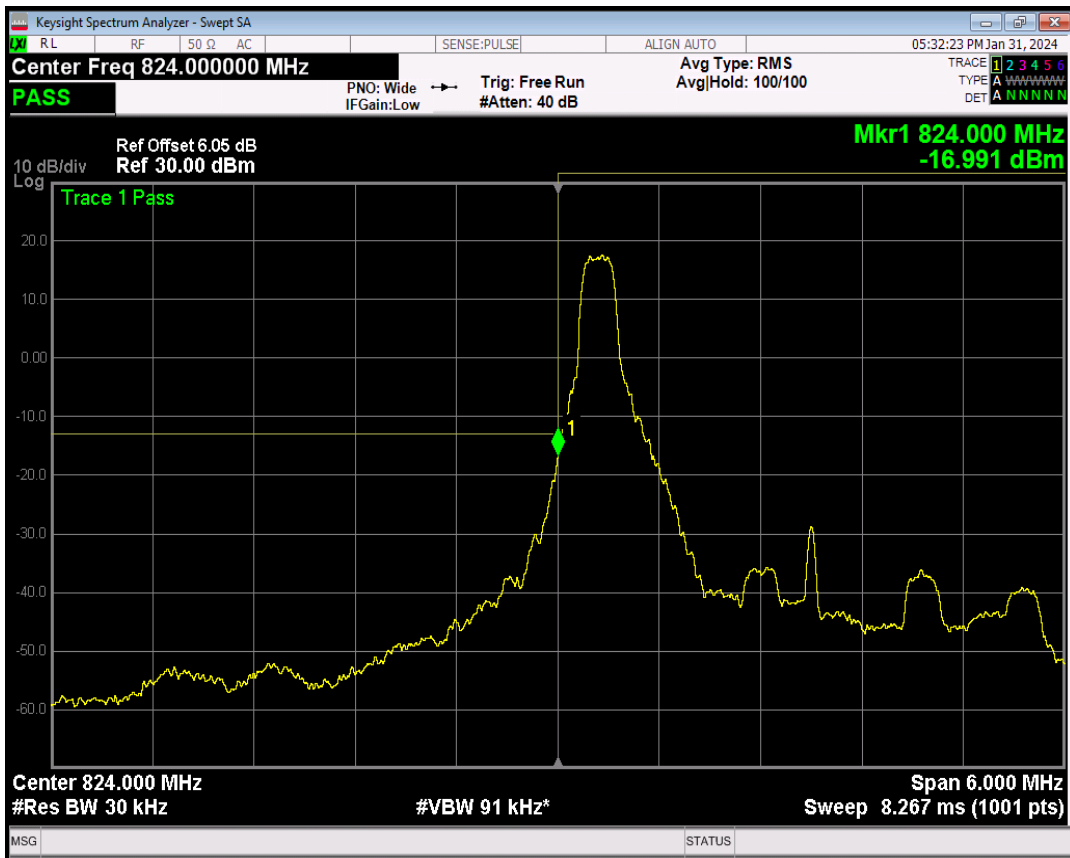
Band5 QPSK BW=3MHz Channel=20415 RB Size=1 Position=#Max
