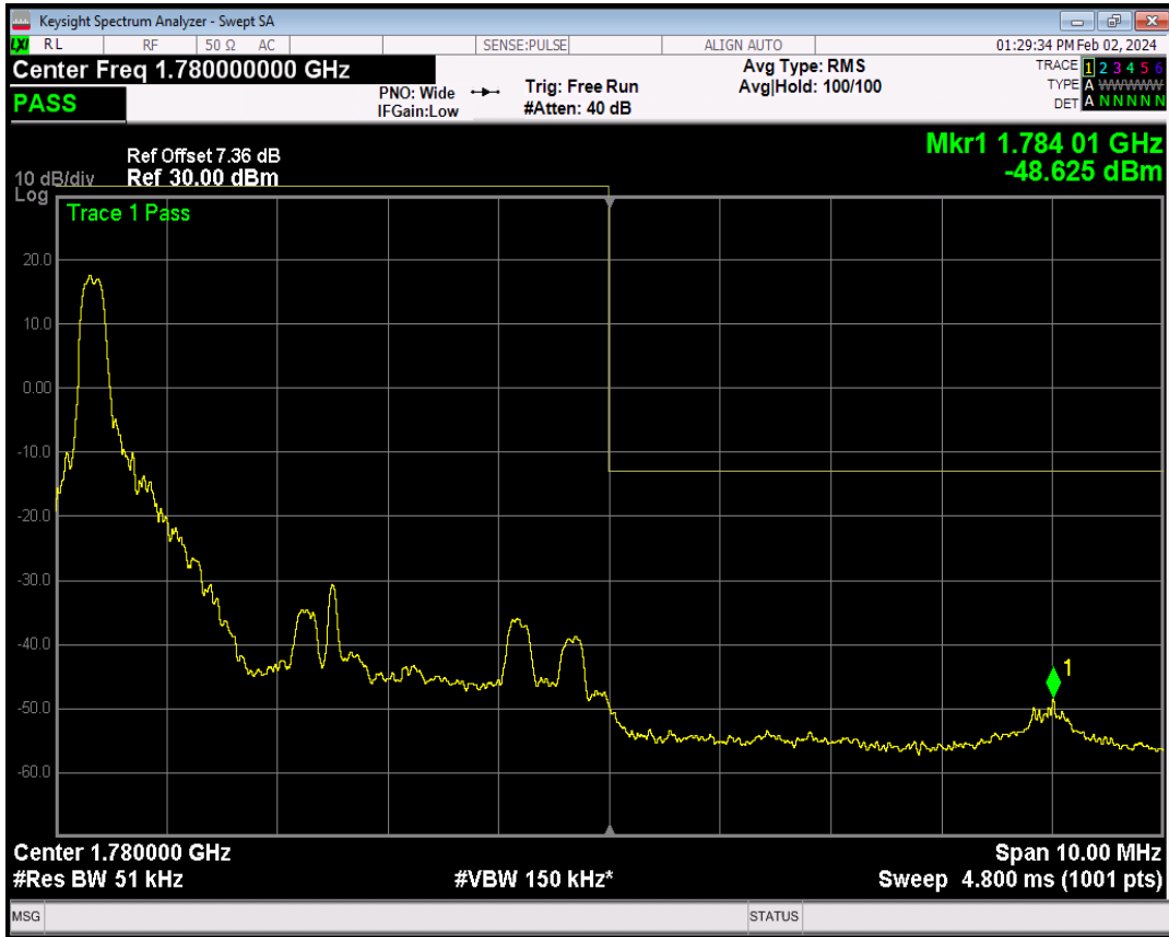
Band66 16QAM BW=5MHz Channel=132647 RB Size=1 Position=#Max
