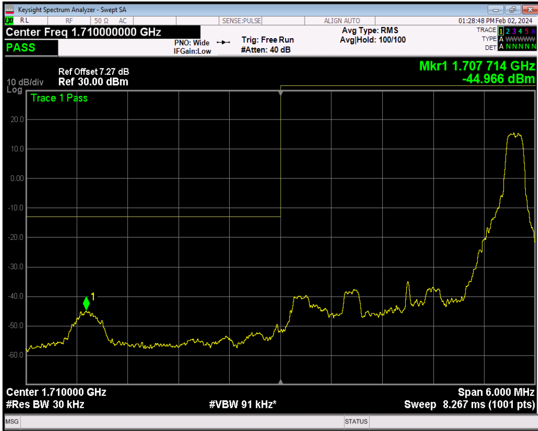
Band66 16QAM BW=3MHz Channel=131987 RB Size=1 Position=#0
