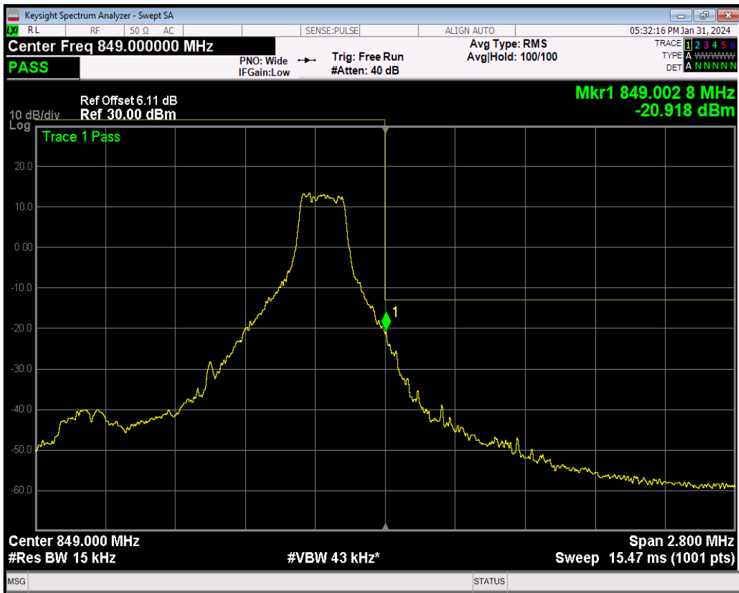
Band5 16QAM BW=1.4MHz Channel=20643 RB Size=6 Position=#0
