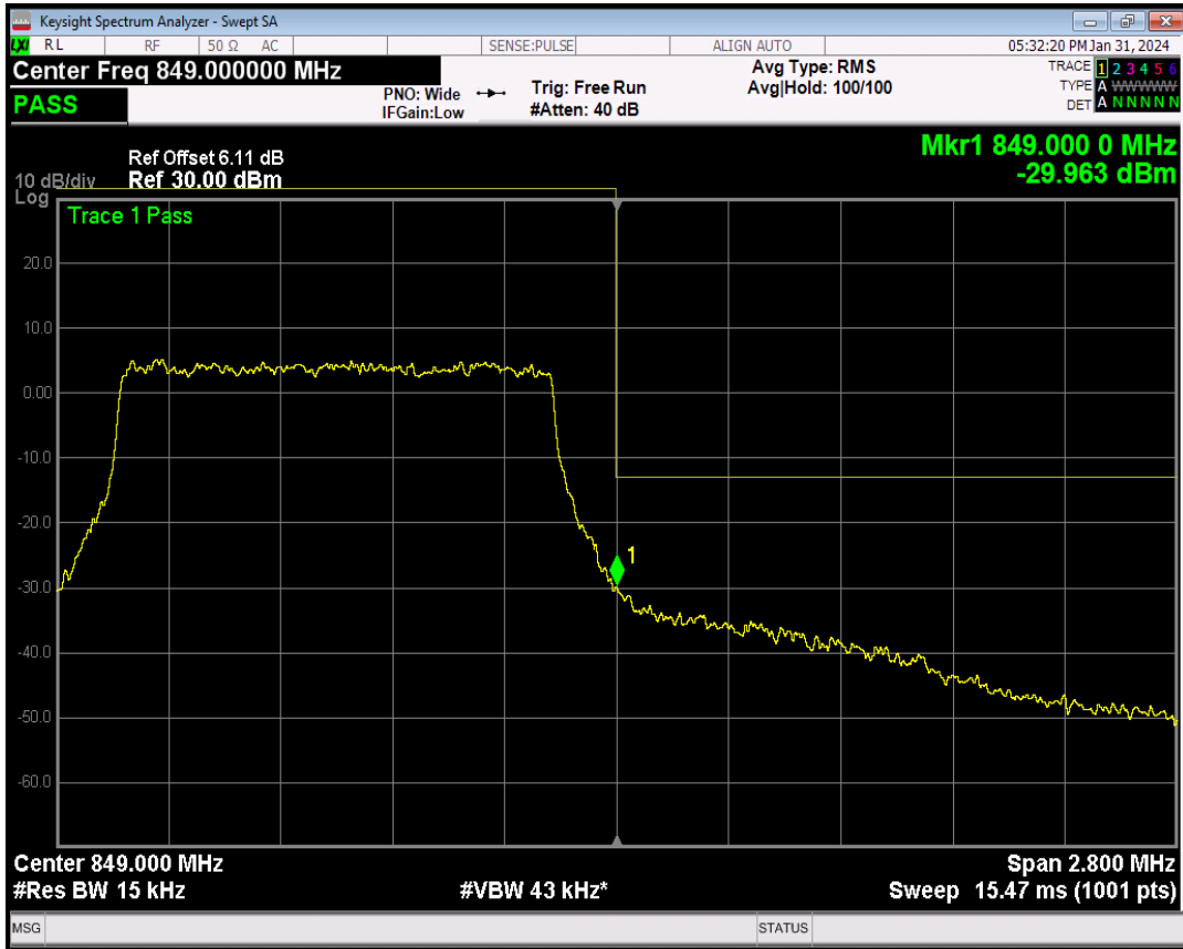
Band5 QPSK BW=3MHz Channel=20415 RB Size=1 Position=#0
