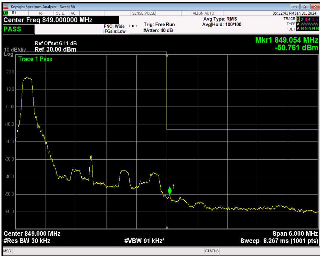
Band5 QPSK BW=3MHz Channel=20635 RB Size=1 Position=#Max
