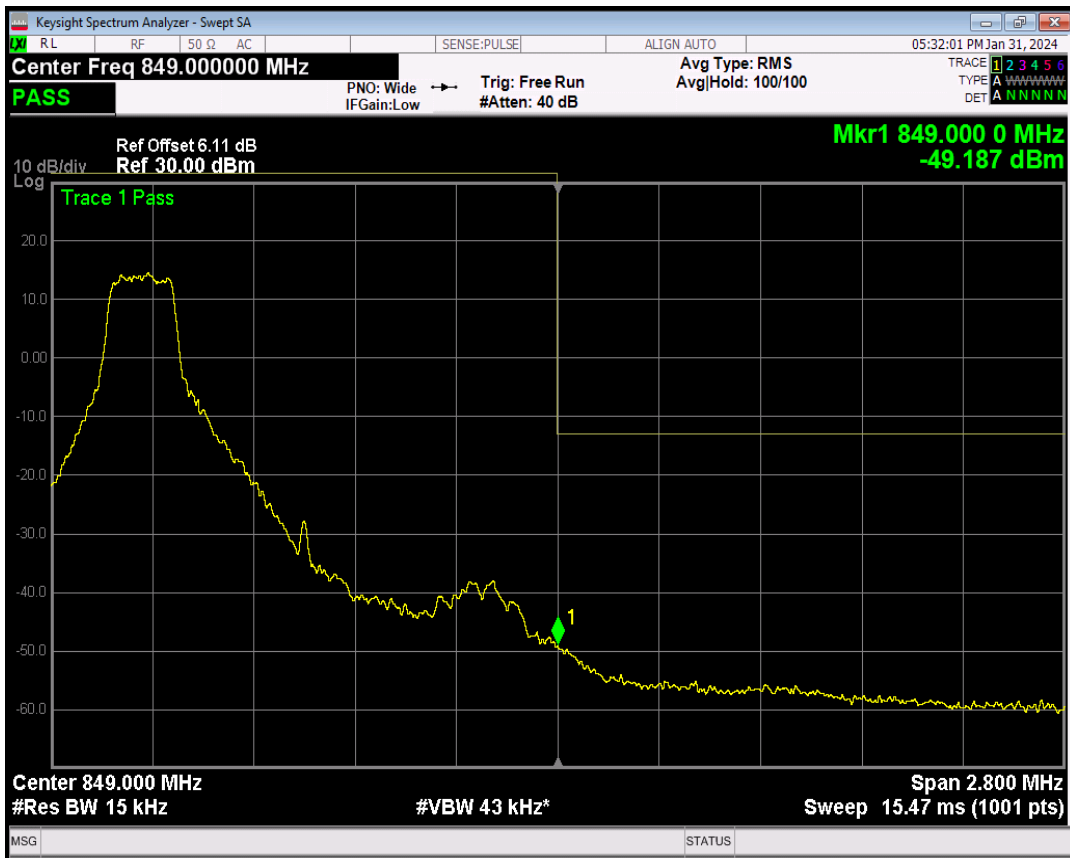
Band5 QPSK BW=1.4MHz Channel=20643 RB Size=1 Position=#Max
