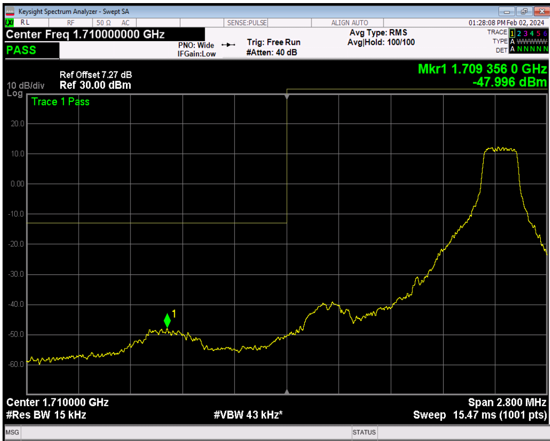
Band66 16QAM BW=1.4MHz Channel=131979 RB Size=6 Position=#0
