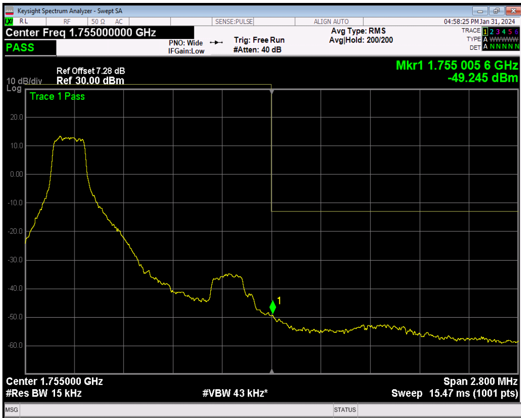
Band4 QPSK BW=1.4MHz Channel=20393 RB Size=1 Position=#Max
