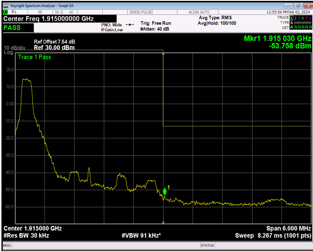
Band25 16QAM BW=3MHz Channel=26675 RB Size=1 Position=#Max
