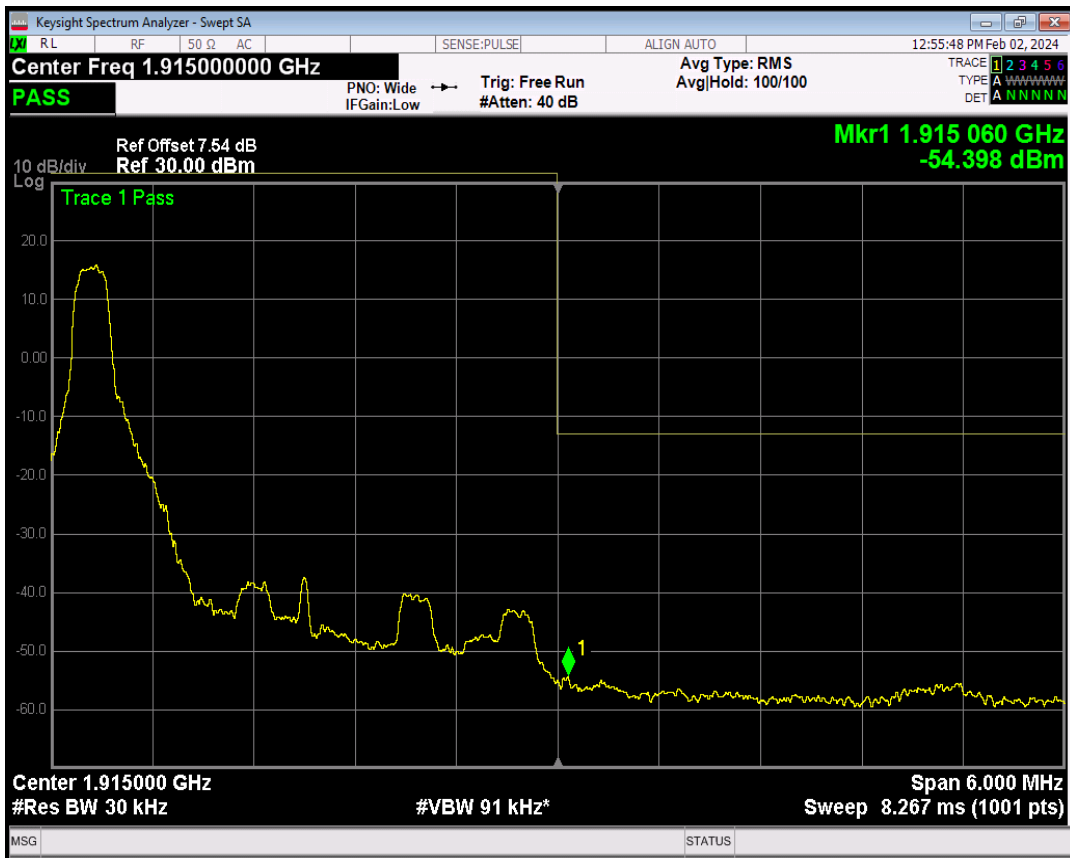
Band25 QPSK BW=3MHz Channel=26675 RB Size=1 Position=#Max
