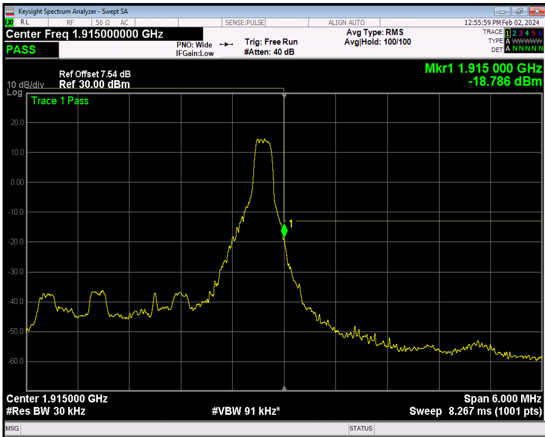
Band25 16QAM BW=3MHz Channel=26675 RB Size=15 Position=#0
