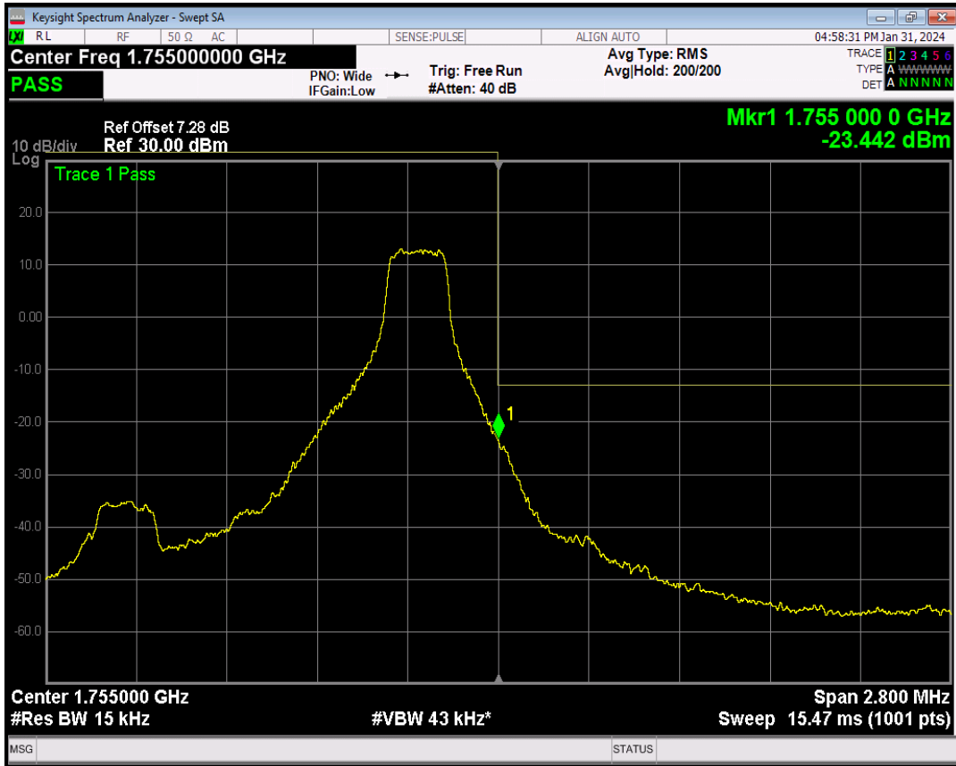
Band4 QPSK BW=1.4MHz Channel=20393 RB Size=6 Position=#0
