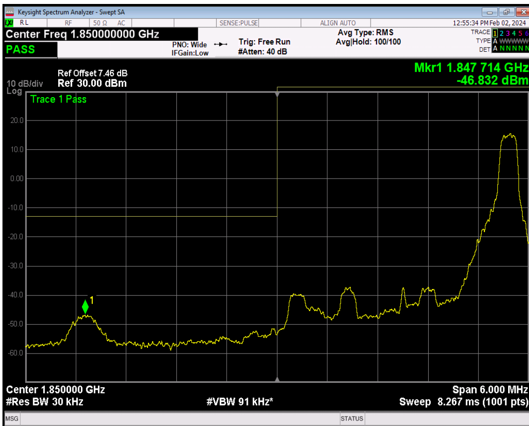
Band25 QPSK BW=3MHz Channel=26055 RB Size=15 Position=#0
