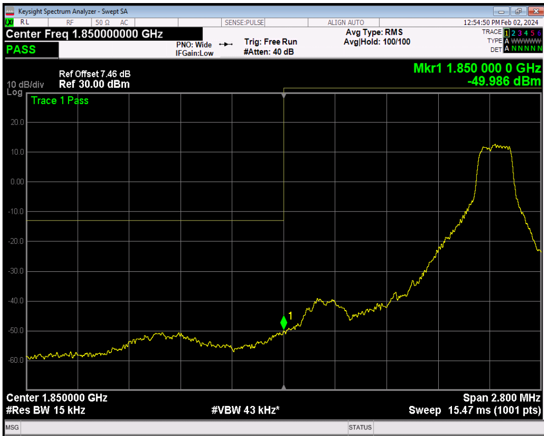
Band25 QPSK BW=1.4MHz Channel=26047 RB Size=1 Position=#0
