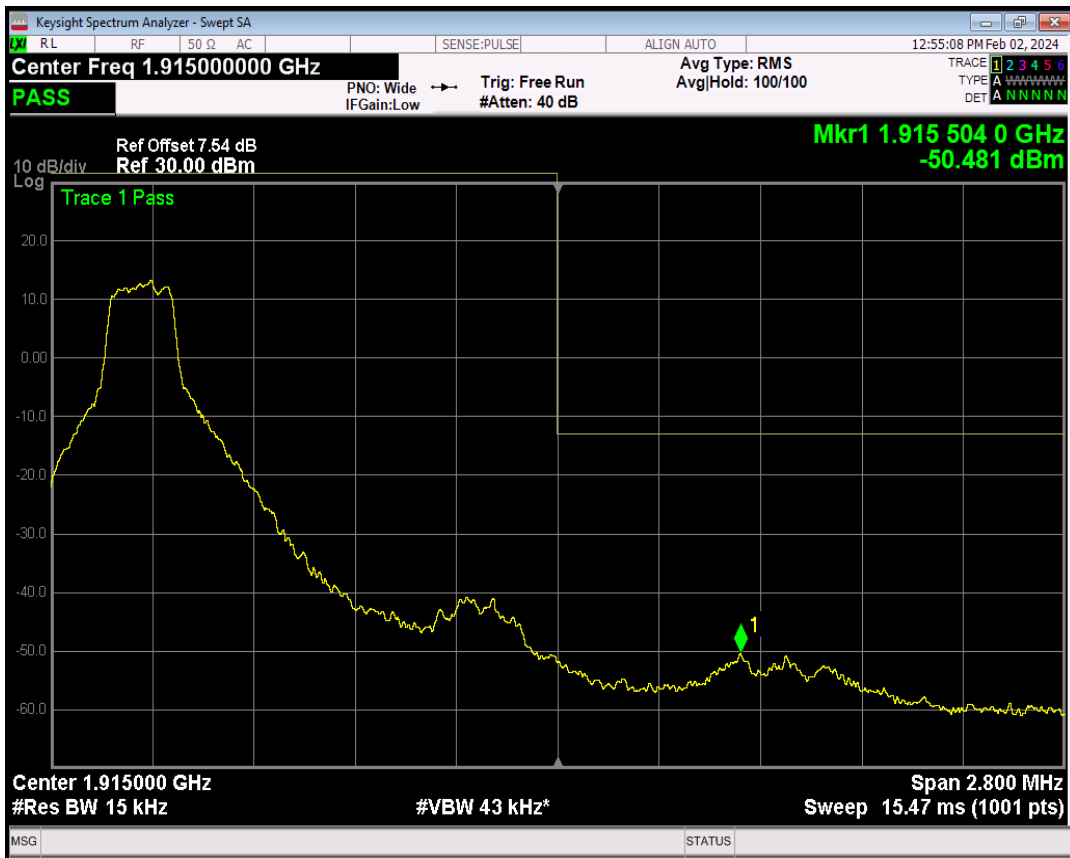
Band25 QPSK BW=1.4MHz Channel=26683 RB Size=1 Position=#Max
