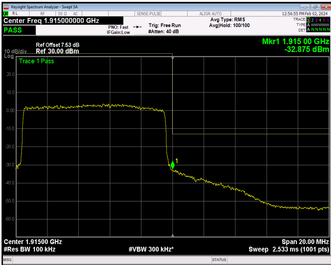
Band25 16QAM BW=10MHz Channel=26640 RB Size=1 Position=#0
