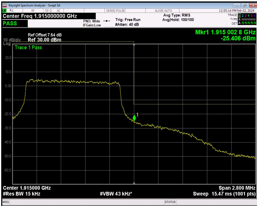
Band25 16QAM BW=1.4MHz Channel=26683 RB Size=1 Position=#0
