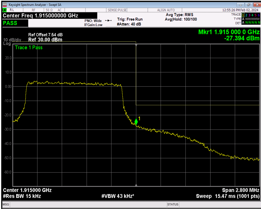
Band25 QPSK BW=3MHz Channel=26055 RB Size=1 Position=#0
