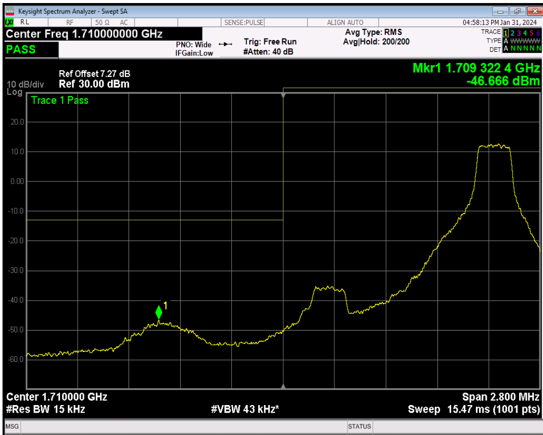
Band4 16QAM BW=1.4MHz Channel=19957 RB Size=6 Position=#0
