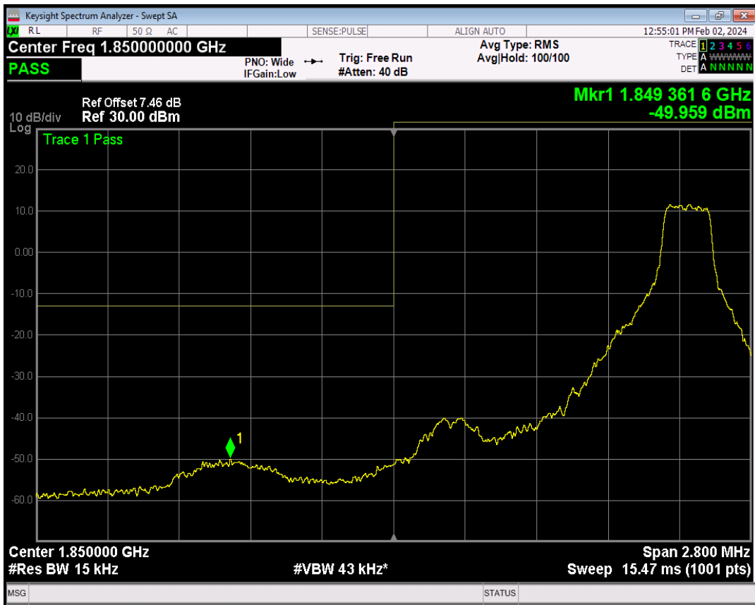
Band25 16QAM BW=1.4MHz Channel=26047 RB Size=6 Position=#0
