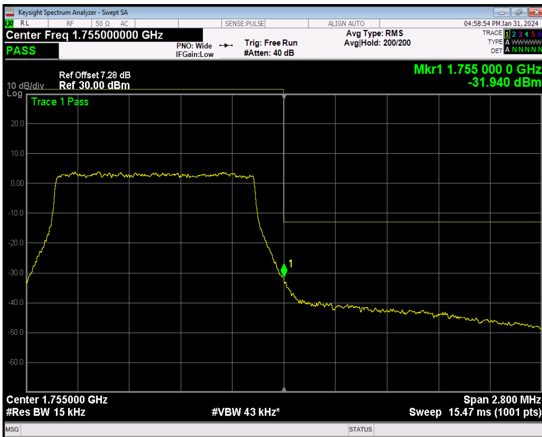
Band4 QPSK BW=3MHz Channel=19965 RB Size=1 Position=#0
