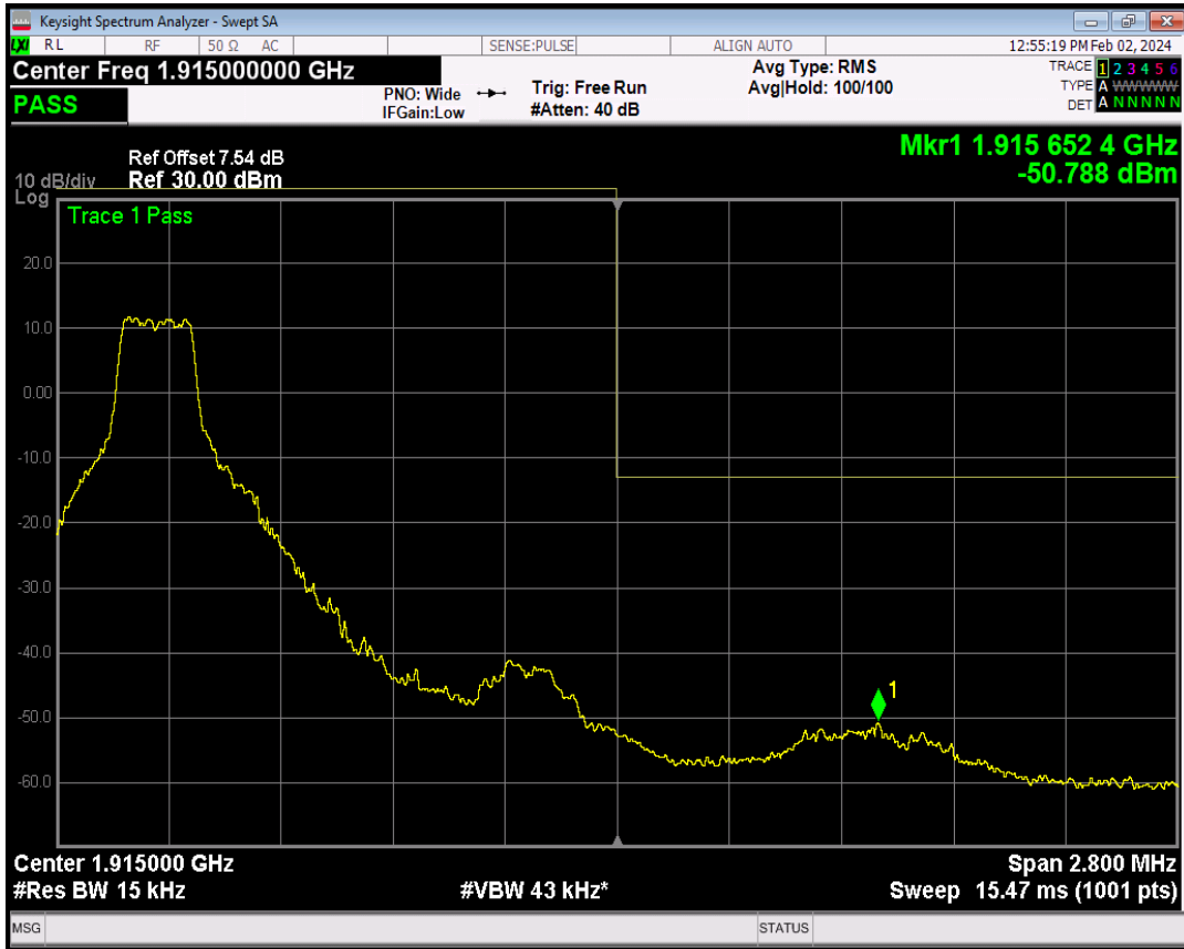
Band25 16QAM BW=1.4MHz Channel=26683 RB Size=1 Position=#Max
