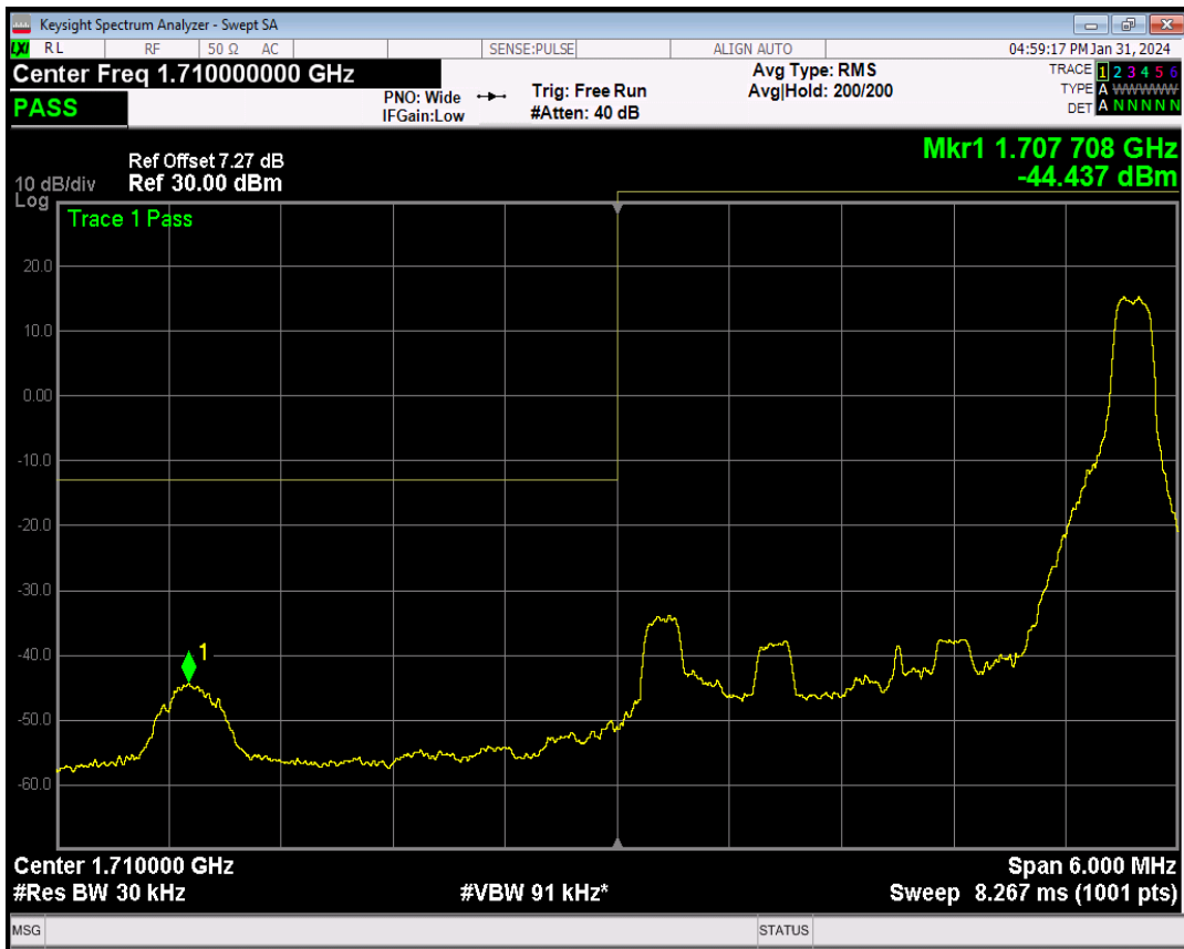
Band4 16QAM BW=3MHz Channel=19965 RB Size=15 Position=#0
