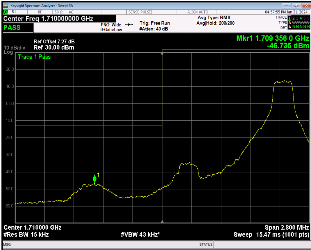
Band4 QPSK BW=1.4MHz Channel=19957 RB Size=6 Position=#0
