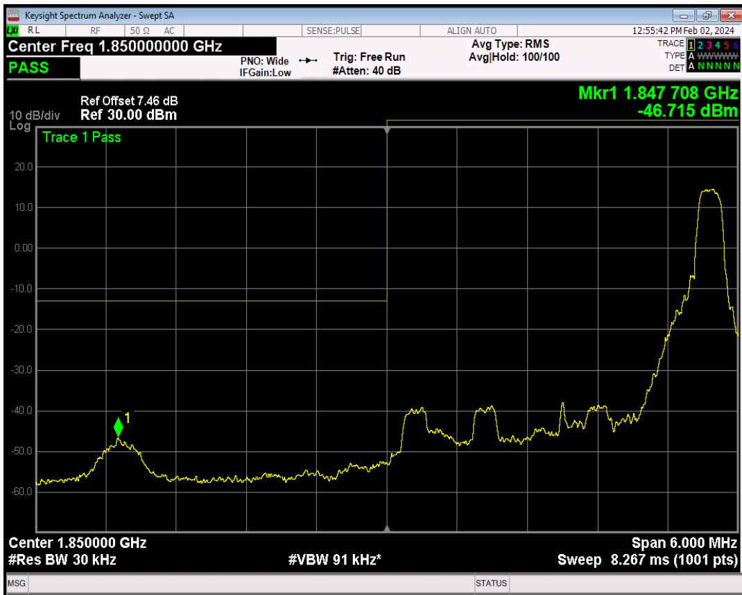
Band25 16QAM BW=3MHz Channel=26055 RB Size=15 Position=#0
