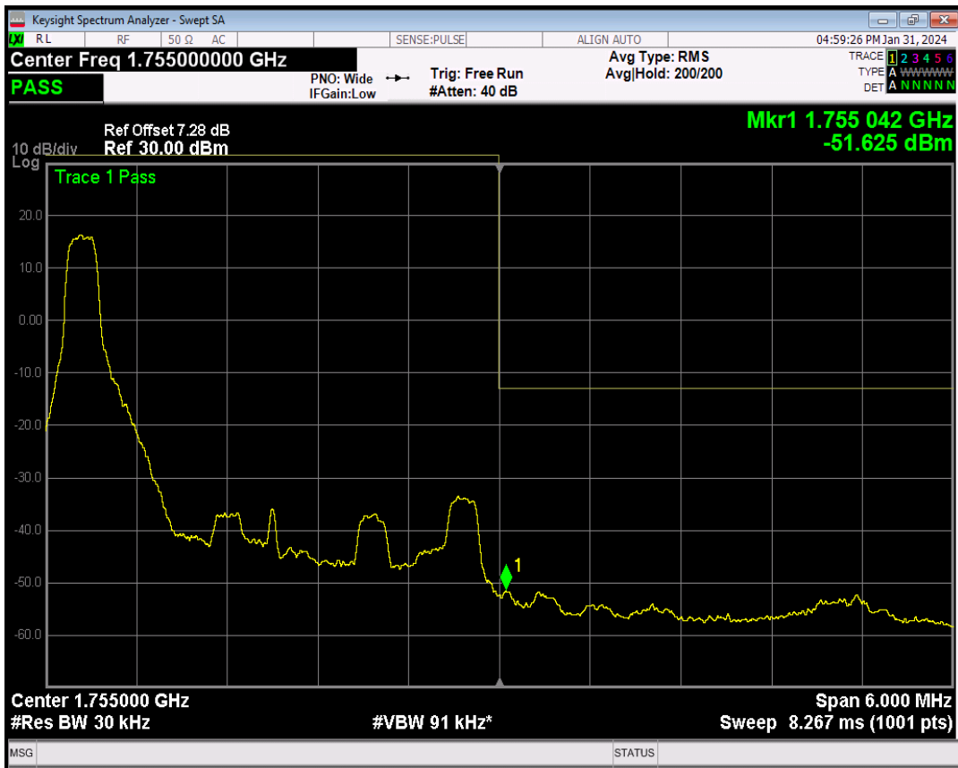
Band4 QPSK BW=3MHz Channel=20385 RB Size=1 Position=#Max
