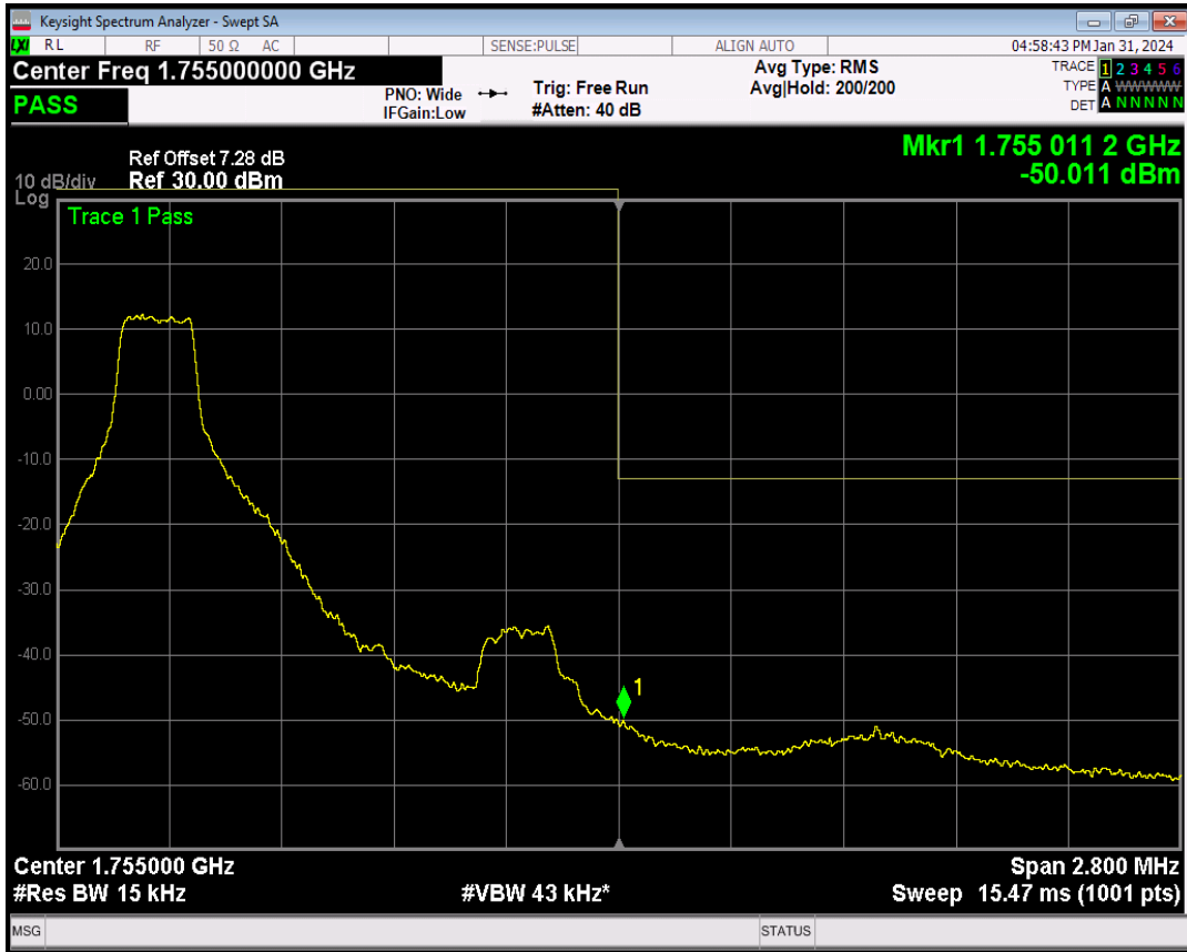
Band4 16QAM BW=1.4MHz Channel=20393 RB Size=1 Position=#Max
