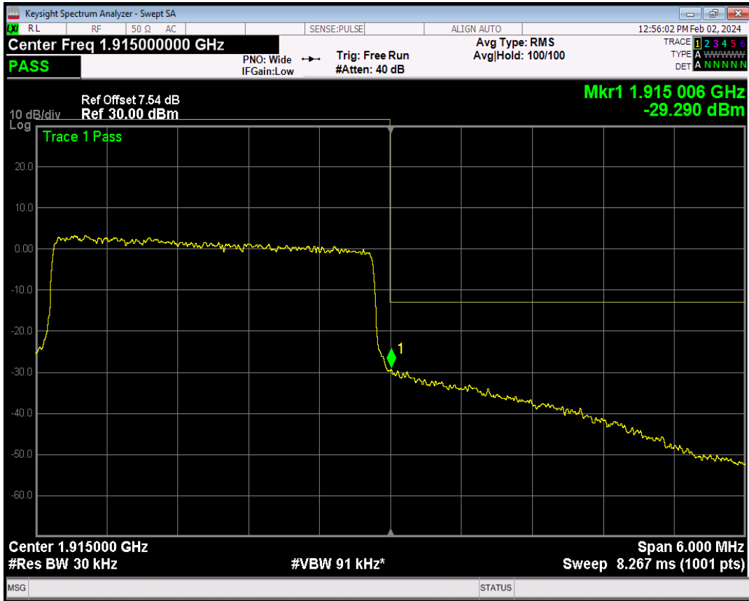
Band25 QPSK BW=5MHz Channel=26065 RB Size=1 Position=#0
