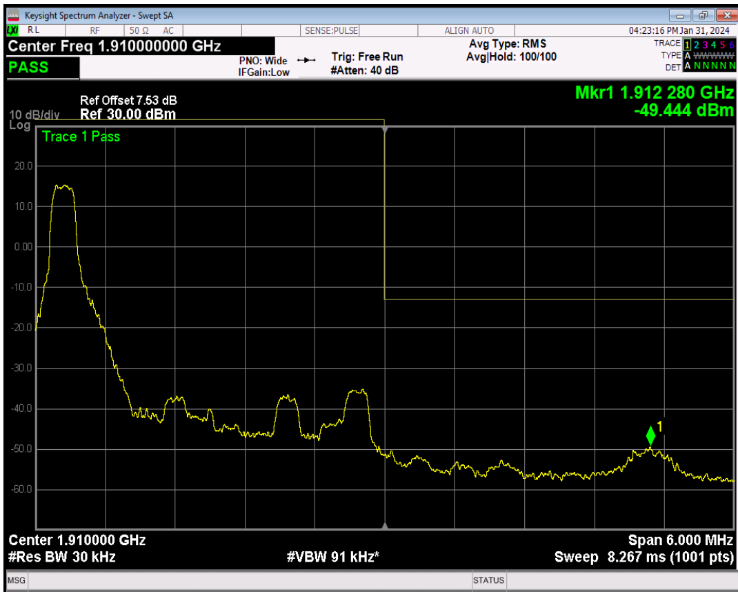
Band2 QPSK BW=3MHz Channel=19185 RB Size=1 Position=#Max
