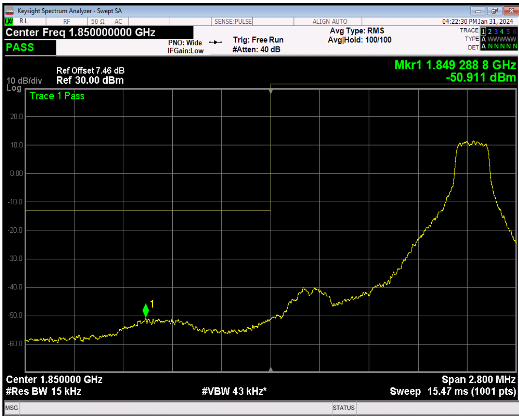
Band2 16QAM BW=1.4MHz Channel=18607 RB Size=6 Position=#0
