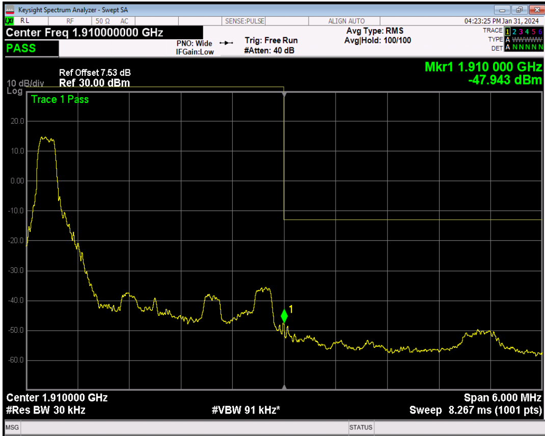
Band2 16QAM BW=3MHz Channel=19185 RB Size=1 Position=#Max
