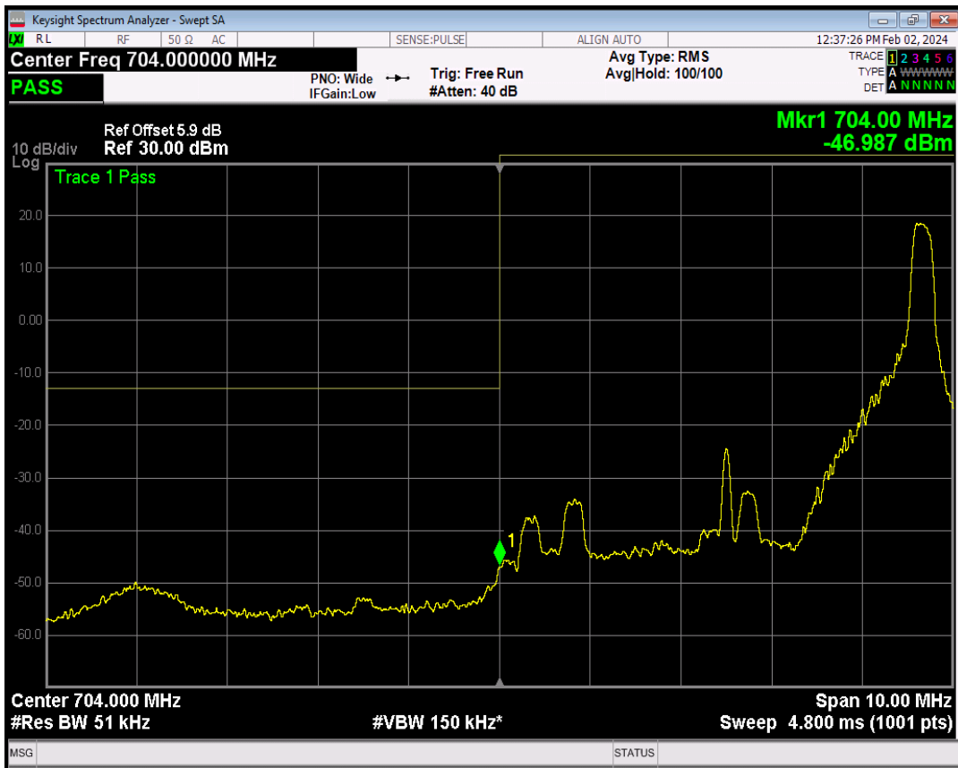
Band17 16QAM BW=5MHz Channel=23755 RB Size=25 Position=#0
