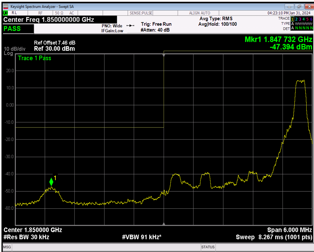
Band2 16QAM BW=3MHz Channel=18615 RB Size=15 Position=#0
