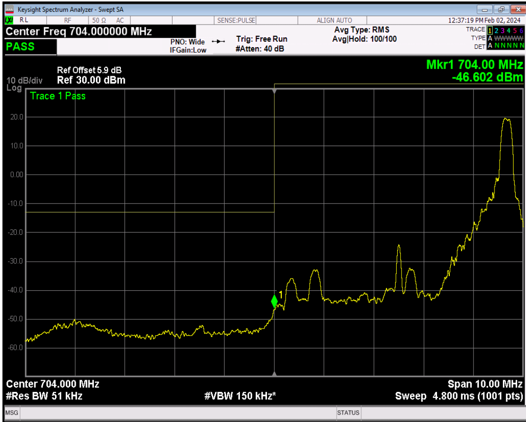
Band17 QPSK BW=5MHz Channel=23755 RB Size=25 Position=#0
