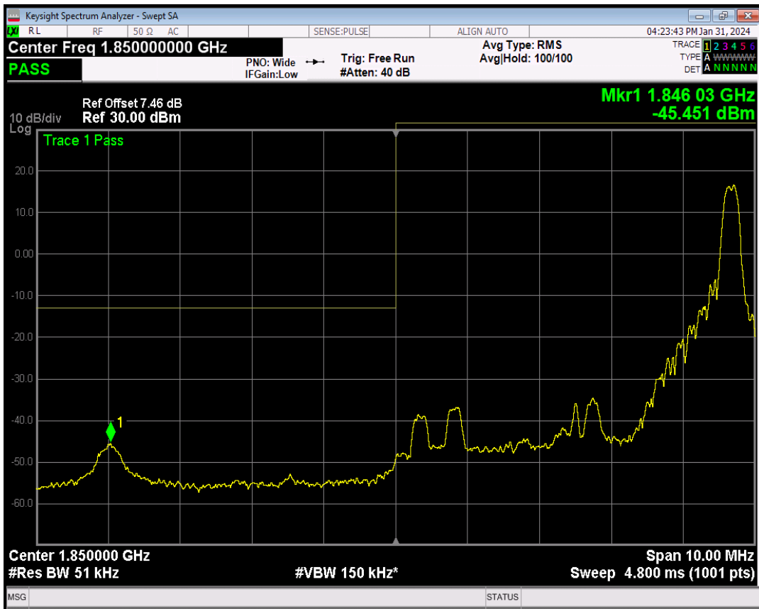
Band2 16QAM BW=5MHz Channel=18625 RB Size=25 Position=#0
