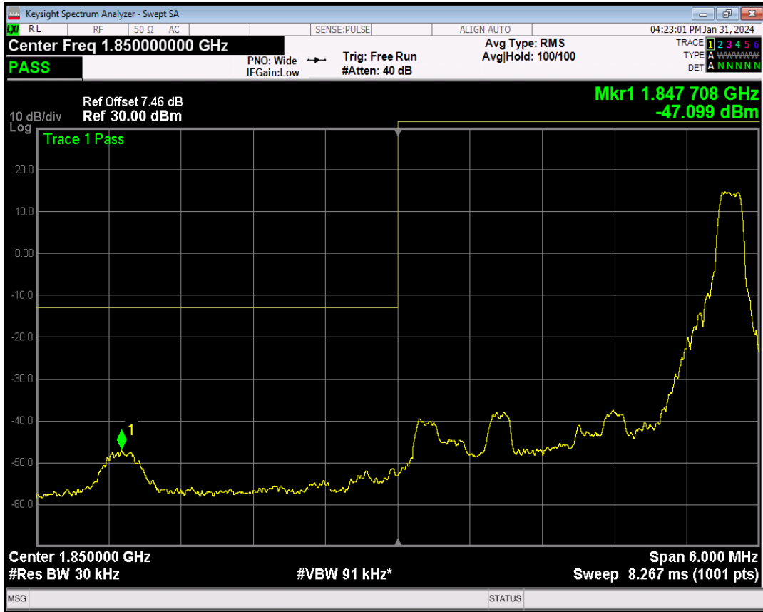
Band2 QPSK BW=3MHz Channel=18615 RB Size=15 Position=#0
