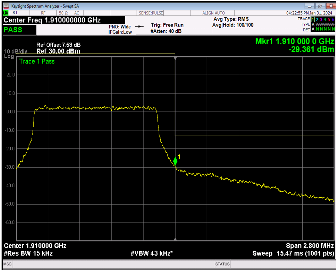
Band2 QPSK BW=3MHz Channel=18615 RB Size=1 Position=#0
