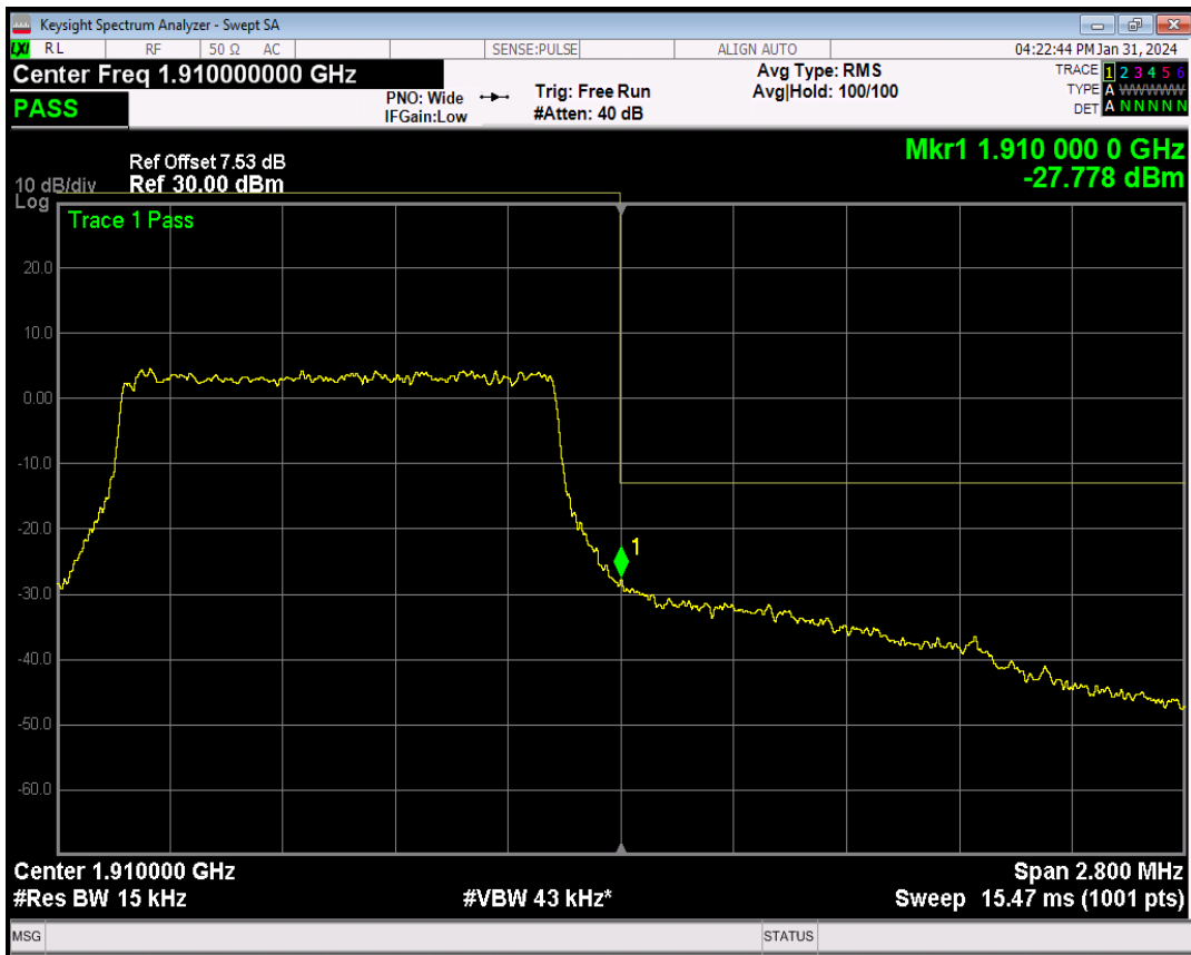
Band2 16QAM BW=1.4MHz Channel=19193 RB Size=1 Position=#0
