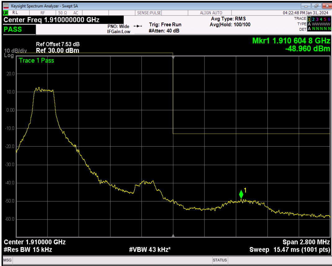
Band2 16QAM BW=1.4MHz Channel=19193 RB Size=1 Position=#Max
