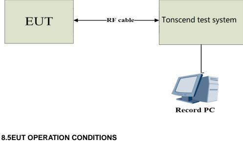
The EUT was programmed to be in continuously transmitting mode.
