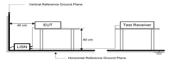
The LISN edge is arranged parallel to the edge of the test table
